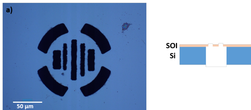
Figure 2.1: The existing geometry of the rectangular trenches on a SOI membrane: Optical image of see-through trenches on SOI/Si substrate (shown in schematic)
