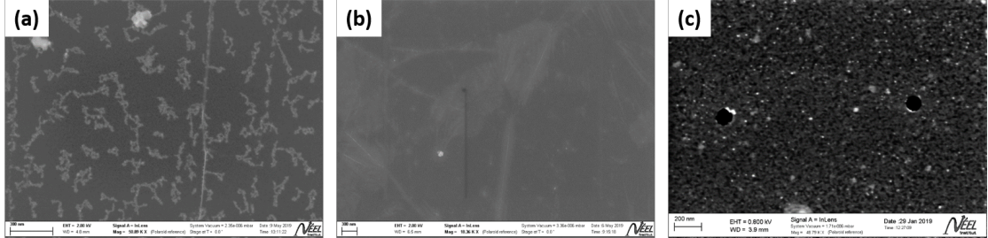
Figure 2.23: Comparison of sample resulting from three different methods (a) annealing with three temperature steps ( 400 °C - 300 °C - 200 °C), (b) annealed at 350 °C and (c) standard process involving as shown in figure 2.17.
