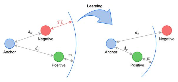
Figure 2.3: Principle of the triplet loss as explained in [SKP15].
