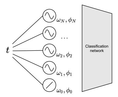
Figure 3.6: Scalar timestamps classification pipeline as proposed in [KGE<sup>+</sup>19]
