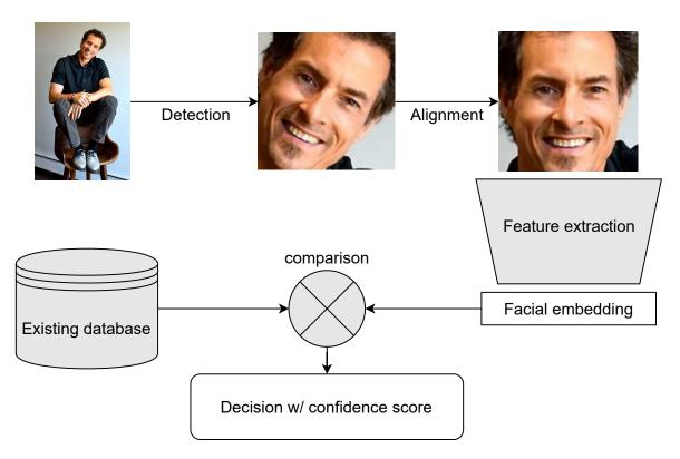
Figure 2.4: Common face recognition model pipeline.
