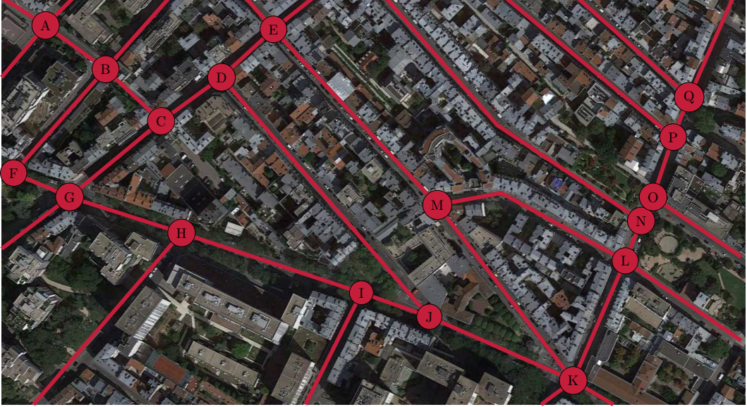
Figure 5.1: Example non-directed graph representing a road network.
