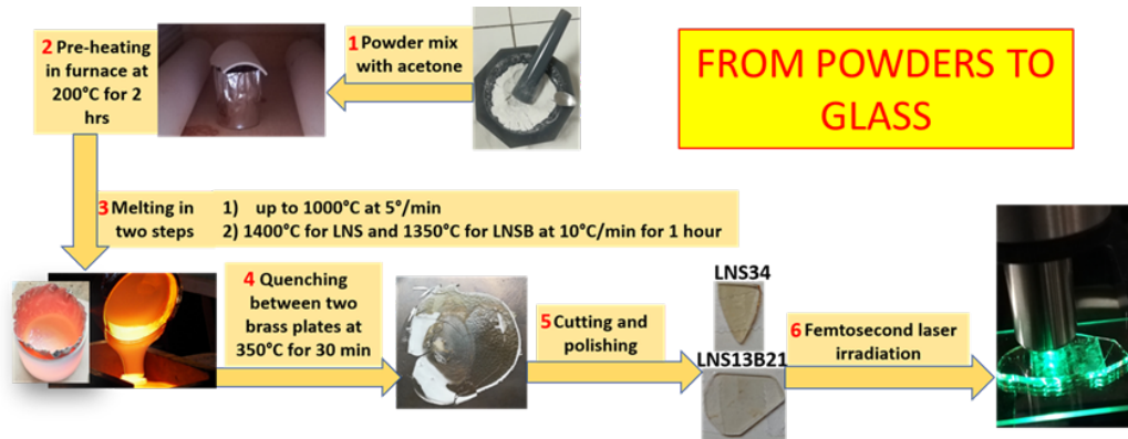
Figure 7: Scheme of glass making process starting from the chemical powders
