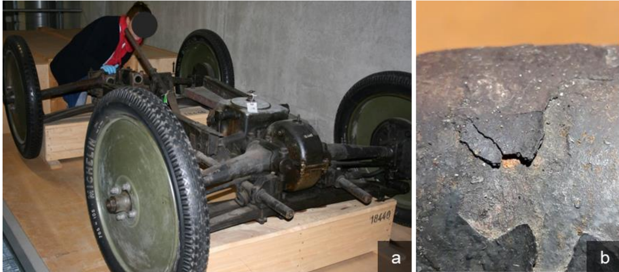
Figure III-8 Photograph of the Châssis (Automobile chassis): full object (a); detail of the paint alteration on the front right axle (b). Dimensions (l x w x h): 2 m x 1.5 m x 1 m.
