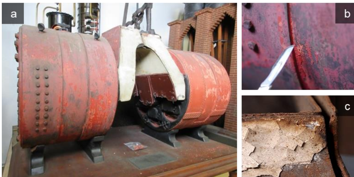
Figure III-3 Photograph of the Chaudière (Model of engine boiler). Dimensions (l x w x h): 90 cm x 60 cm x 60 cm. Surface alteration is shown in images b and c.
