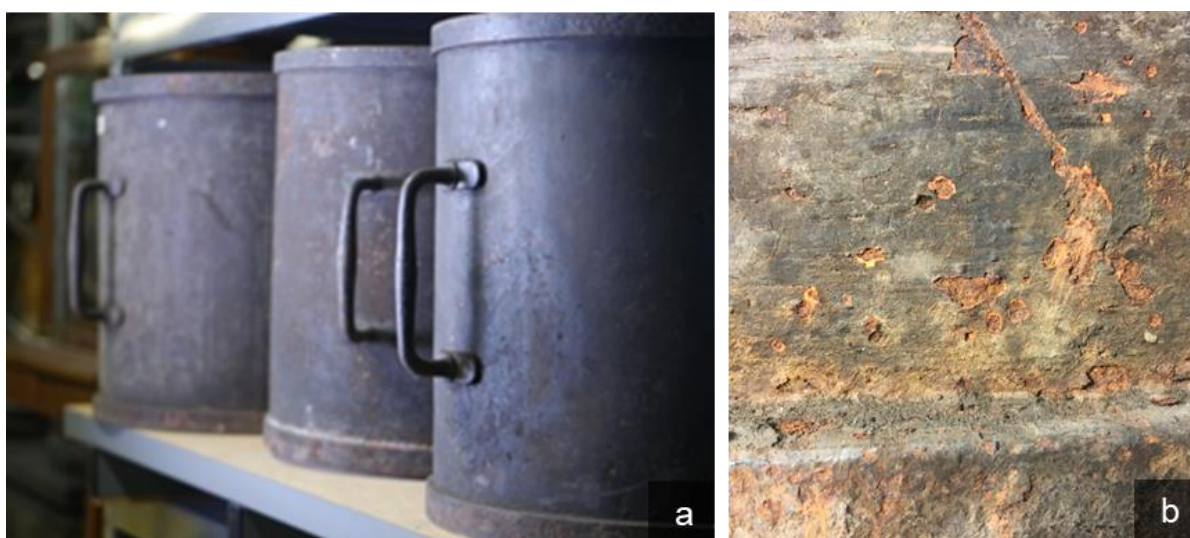
Figure III-4 Photograph of three measures (a) of the Série de 6 mesures (Set of six measuring containers). Dimensions (h x d): 52 cm x 62 cm. Surface alteration with paint loss and corrosion (b).
