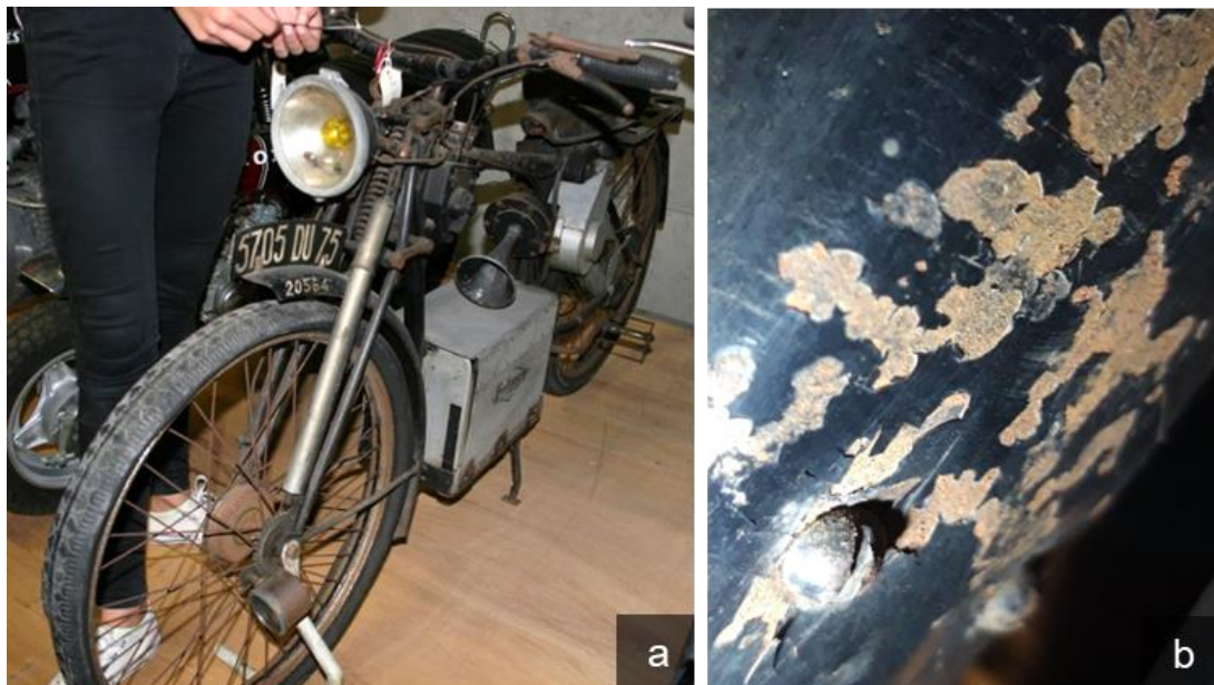
Figure III-9 Photographs of the Vélocoteur (Electric motorbike): full object (a); detail of the paint alteration at the bottom right of the front fender (b). Dimensions (l x w x h): 170 cm x 50 cm x 70 cm.
