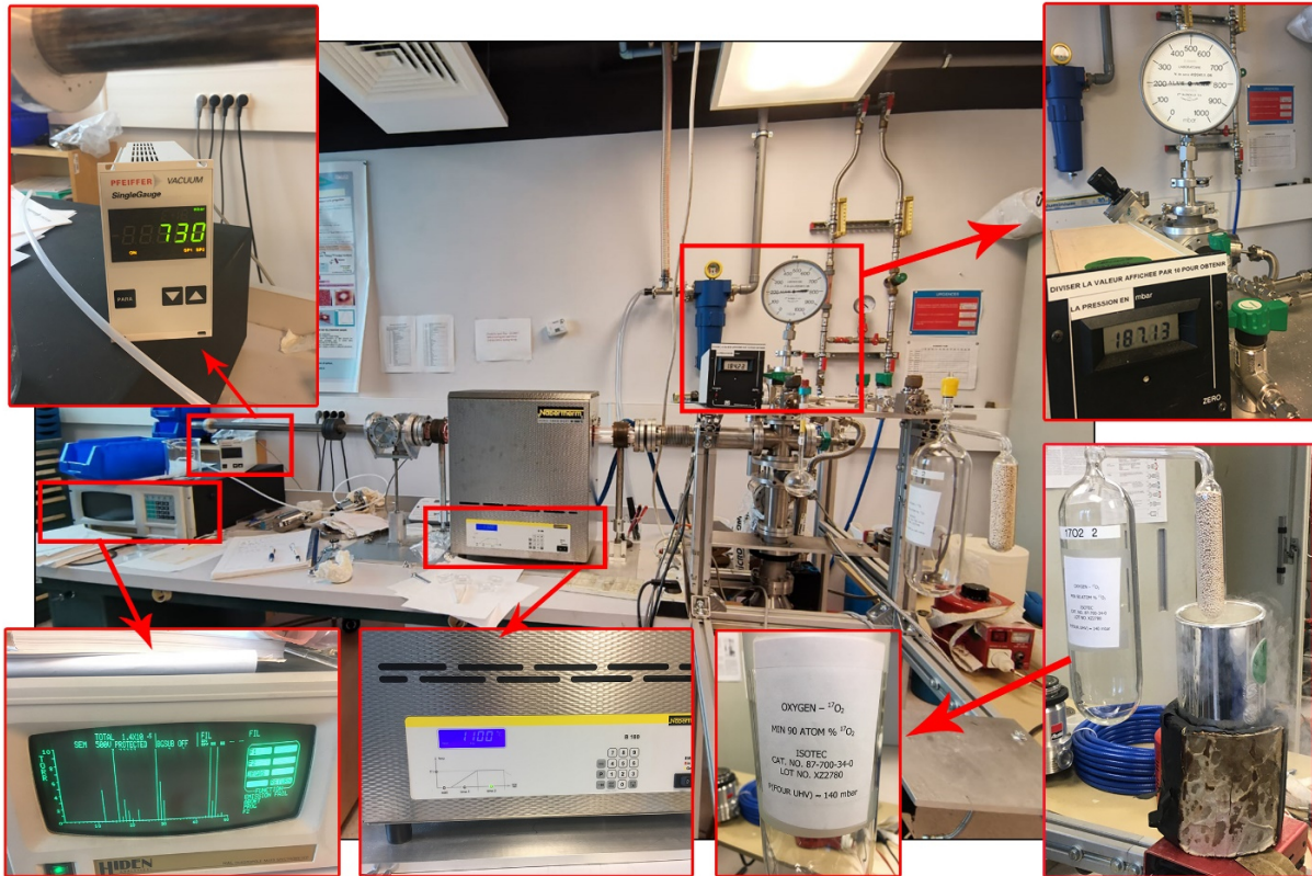
Figure 3.8: Quartz tube furnace equipped for handling isotopically enriched gases, used for ^{17}\text{O} thermal oxide growth on silicon (INSP).
