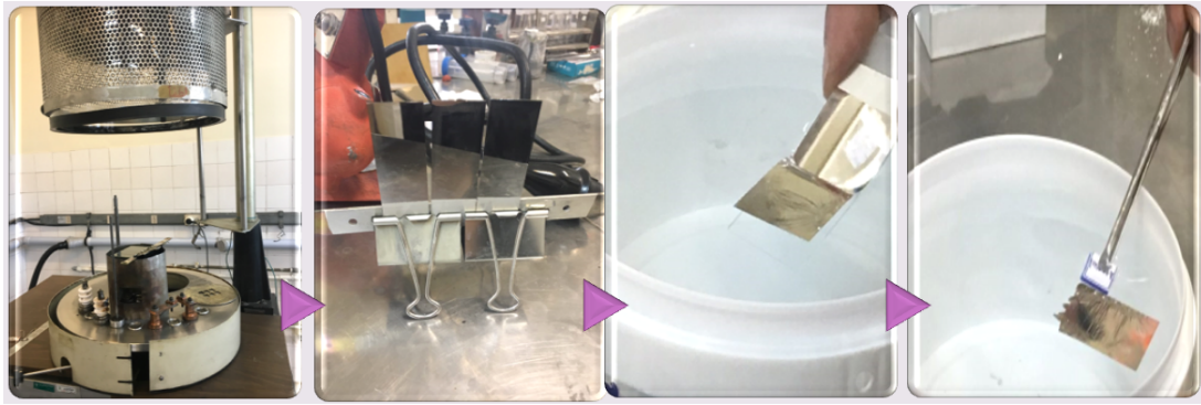
Figure 3.4: Preparation of a thin self-supporting vacuum evaporated Al film (VDGT)
