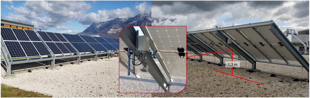
Figure 4.1: INES fixed tilt test bench, France. Left) View of one of the three rows. Right) View from the backside of the first row enhancing the backside reference cell position.
