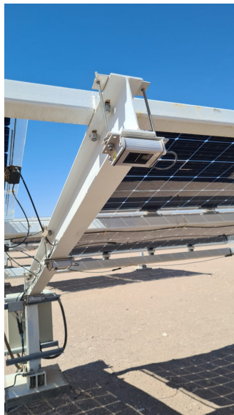
(c) Reference cells at the POA of the fix tilted installation at the PSDA for rear irradiance measurement.
