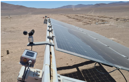
(a) Reference cells in the POA of a fix tilted installation at the PSDA.
