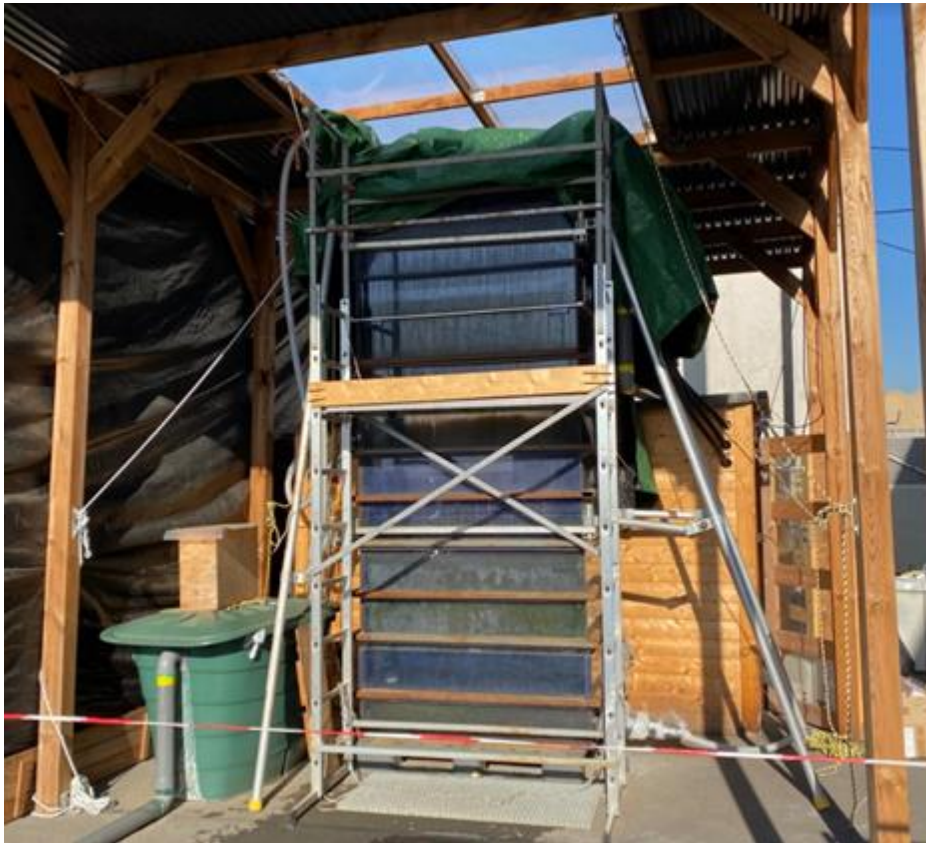
Figure GC.1: Pilot-scale membrane tank used in preliminary tests of accelerated ageing in on-site conditions.
