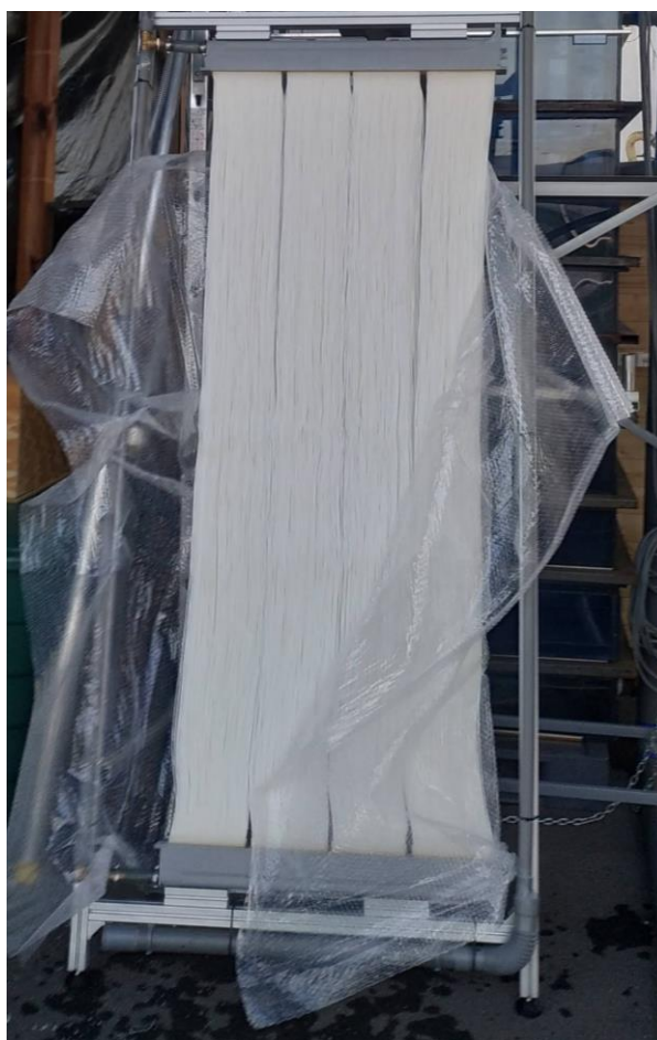
Figure 2.3: ZeeWeed® 500D membrane module.
