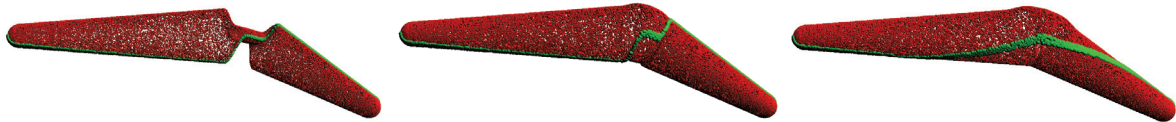
Figure 3.8 – Comparison of skinning approaches on a sphere-mesh model with combined twist and bend motions. Left to right: Isotropic Linear Blend Skinning, Isotropic Skinning with Dual Quaternions, Ours
