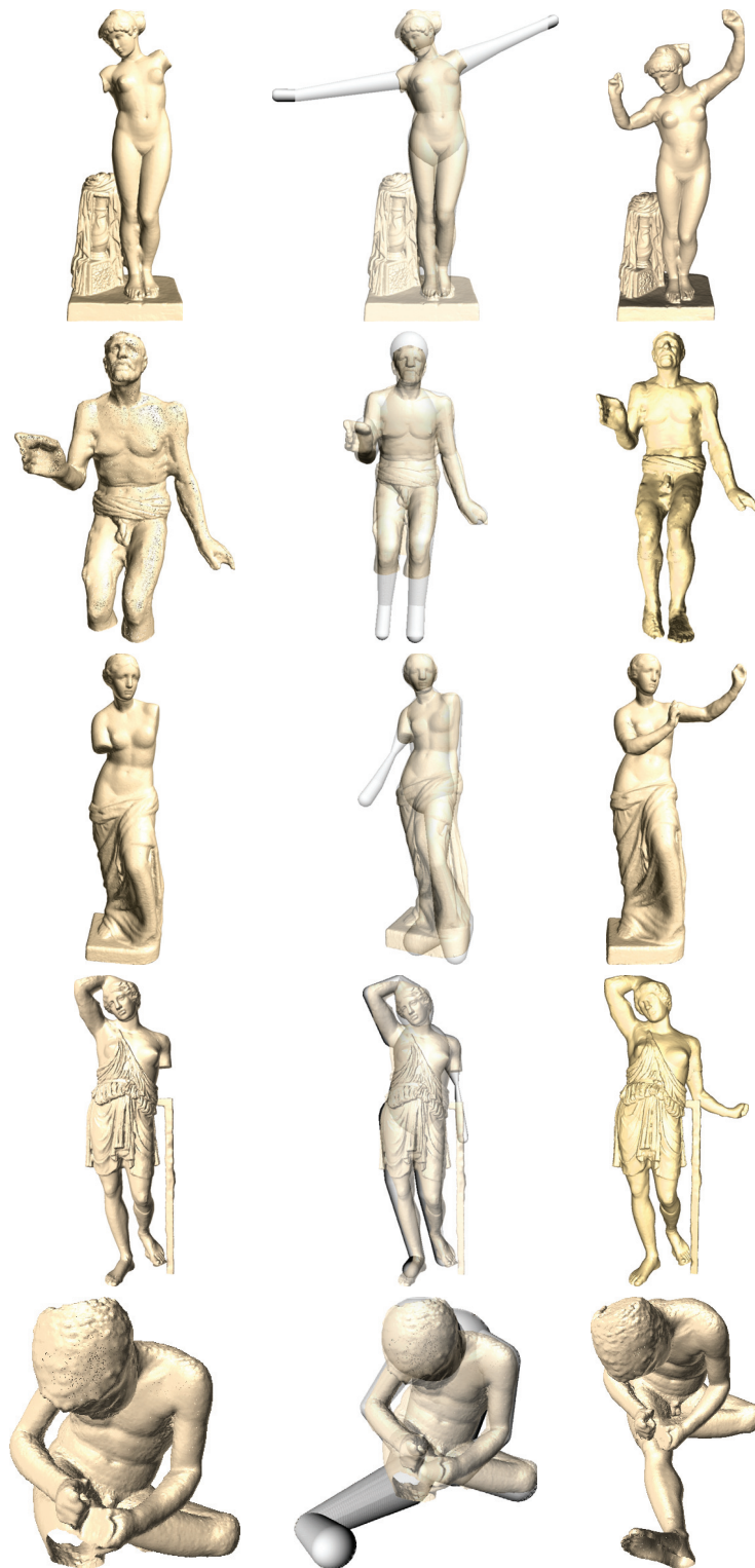
Figure 5.4 – Registration and restoration of 5 incomplete statues, Esquiline Venus (first row), Old Fisherman (second row), Venus de Milo (third row), Wounded Amazon (fourth row) and Spinario (fifth). First column: initial point set, second column: overlay of the registered model and the point set, third column: final restoration.
