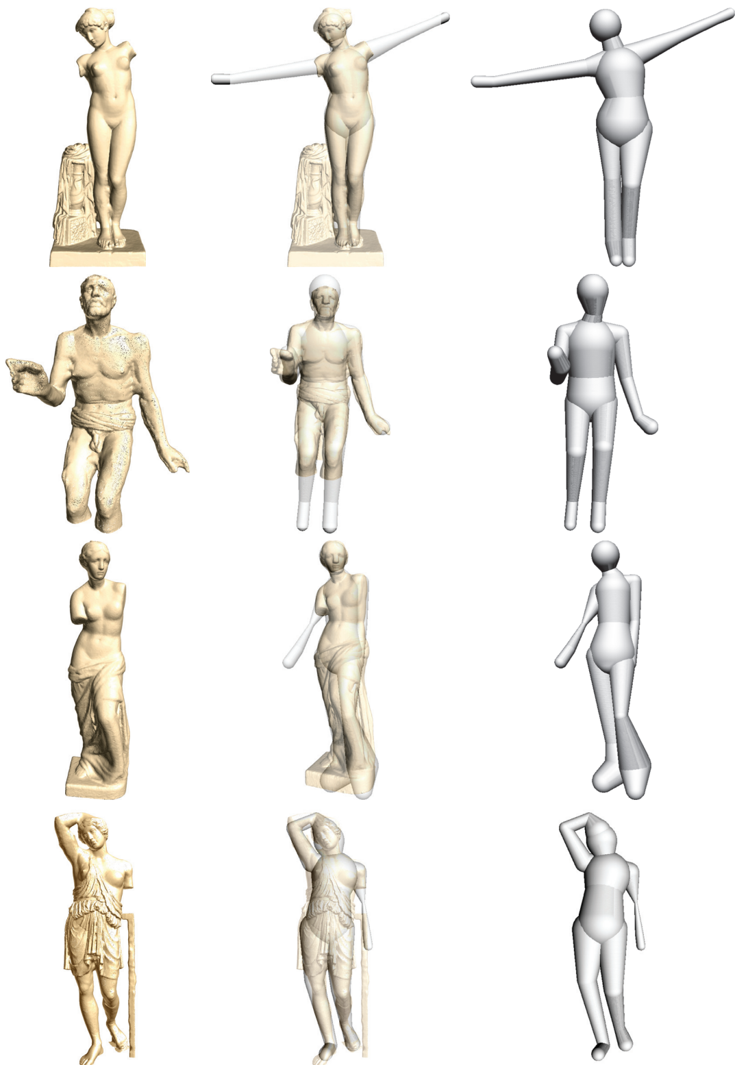
Figure 2.14 – Registration of 4 incomplete statues, Esquiline Venus (first row), Old Fisherman (second row), Venus de Milo (third row) and Wounded Amazon (fourth row). First column: initial point set, second column: overlay of the registered model and the point set, third column: registered model alone.
