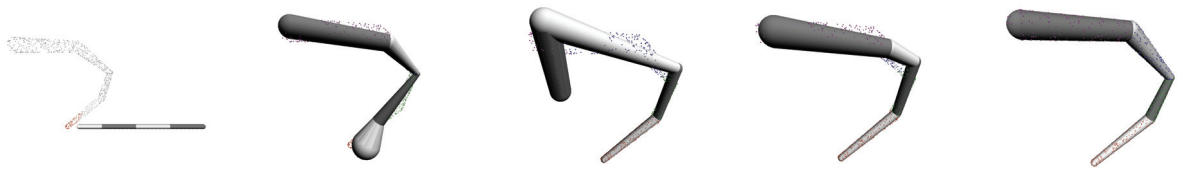
Figure 2.21 – Simultaneous Optimization for a chain of bones applied after the first Fakir forward pass. From left to right: initial position (after our forward step), position after 10 iterations, position after 35 iterations, position after convergence (43 iterations).
