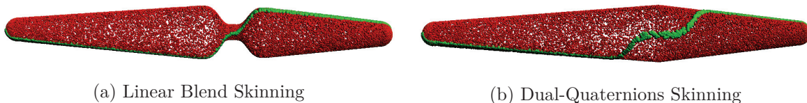
Figure 3.6 – Twist motion: near blend Skinning and Dual-Quaternions Skinning to be compared with our approach in figure 3.7 that uses twist specific weights. Green dots show points that were aligned before the twisting rotation.
