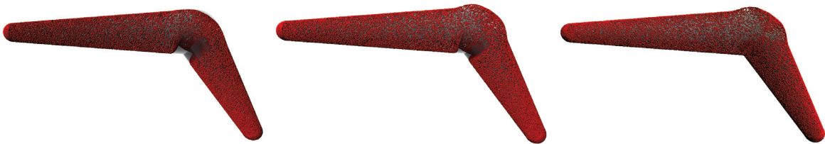
(a) Linear blend skinning (b) Dual Quaternions skinning (c) Our anisotropic skinning
