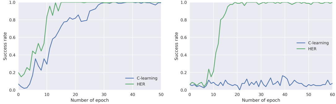
(b) Comparing HER and the C-learning update, both together with DDPG, implemented in an HER open-source implementation (Dai, 2019) we also used for our \delta -DQN implementation. In the FetchReach environment (Left), both HER and C-learning are able to learn (as \delta -DQN, see figure 16.1). In FetchPush (right), the next environment in the OpenAI suite (Plappert et al., 2018), HER is able to learn while C-learning is not (as \delta -DQN, see Section 16.4). Hence, in that setting, there is no significant difference between \delta -DQN and C-learning.
