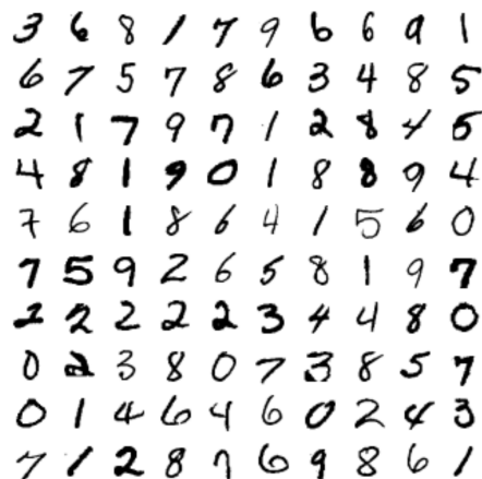
Figure 1.1 – Examples taken from the MNIST data set. Since the image are grayscale, the dimension D of the data is their number of pixels, which is D = 28 \times 28 = 784 . Source: [LBBH98, Fig 4].
