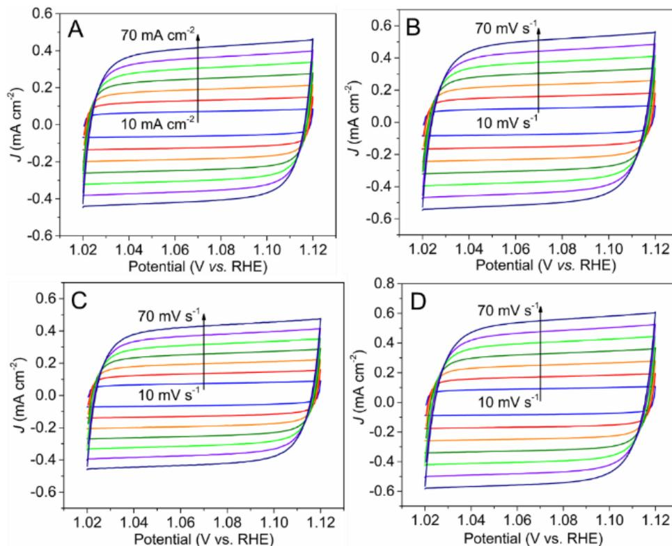
Figure 15. The CV curves in the potential range of 1.02-1.12 V vs. RHE with various scan rates in  $N_2$ -saturated 0.1 M KOH solution of (A)  $^{1.15}Fe@NGC/CB$ ; (B)  $^{4.5}Fe@NGC/CB$ ; (C)  $^{16.2}Fe@NGC/CB$ ; (D)  $^{4.5}Fe@NGC/CB-AL$
