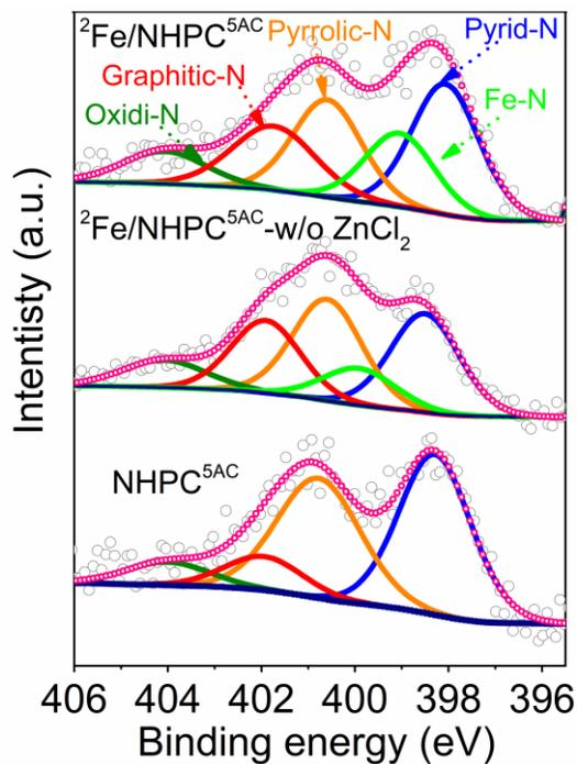
Figure 11. High resolution XPS N 1s core level region of <sup>2</sup>Fe/NHPC<sup>5AC</sup>, <sup>2</sup>Fe/NHPC<sup>5AC</sup>-w/o ZnCl<sub>2</sub>, and NHPC<sup>5AC</sup>.
