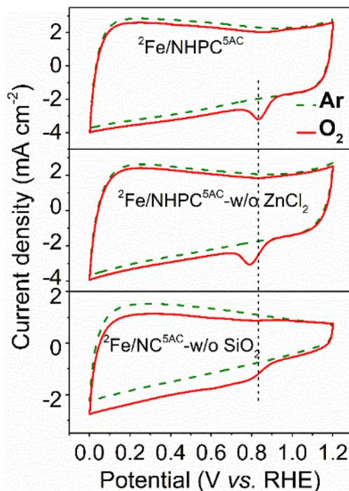
Figure 12. Cyclic voltammetry (CV) curves under Ar and O<sub>2</sub>- saturated 0.1 M KOH solution at scan rate of 50 mV s<sup>-1</sup> for <sup>2</sup>Fe/NHPC<sup>5AC</sup>, <sup>2</sup>Fe/NHPC<sup>5AC</sup>-w/o ZnCl<sub>2</sub>, and <sup>2</sup>Fe/NC<sup>5AC</sup>-w/o SiO<sub>2</sub>.
