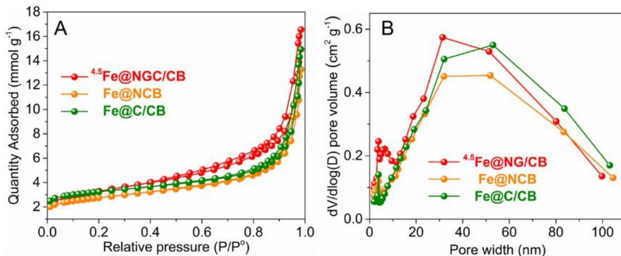
Figure 5. (A)  $\text{N}_2$  adsorption-desorption isotherm plots of  $^{4.5}\text{Fe@NGC/CB}$  and control samples without using glucose ( $\text{Fe@NCB}$ ), urea ( $\text{Fe@C/CB}$ ) recorded at 77 K along with (B) the respective pore size distributions (BJH method) based on desorption branch.
