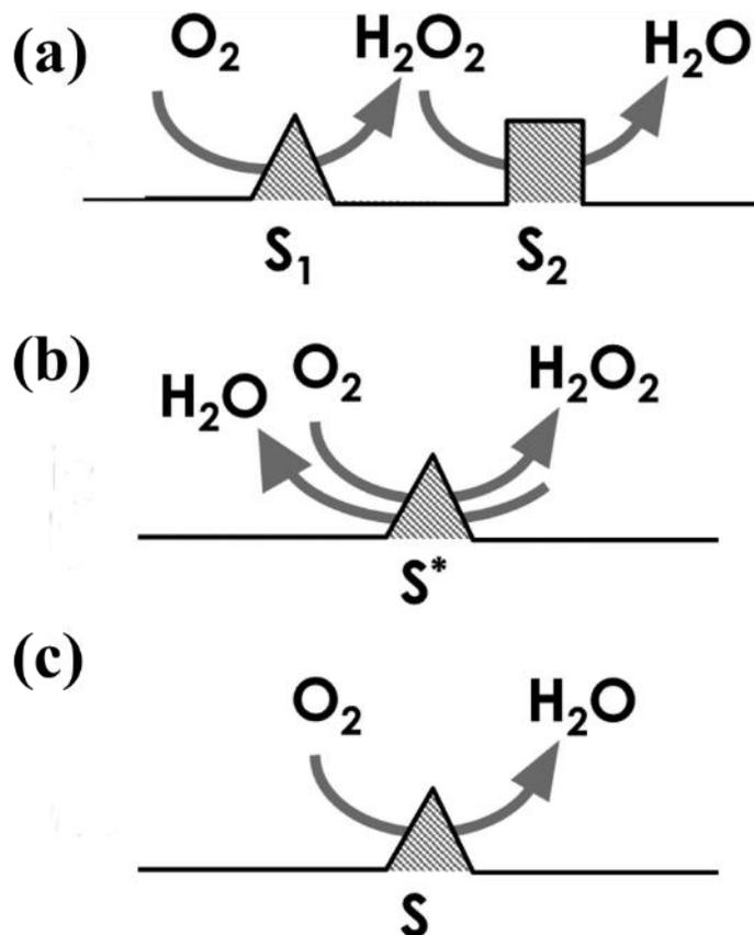
**Figure 3.** Possible reaction pathways and active sites of performing the ORR process. (a) dual site  $2 \times 2 e^-$ , (b) single site  $2 + 2 e^-$ , and (c) single site direct  $4 e^-$  mechanism. Reproduced from Ref. [64]
