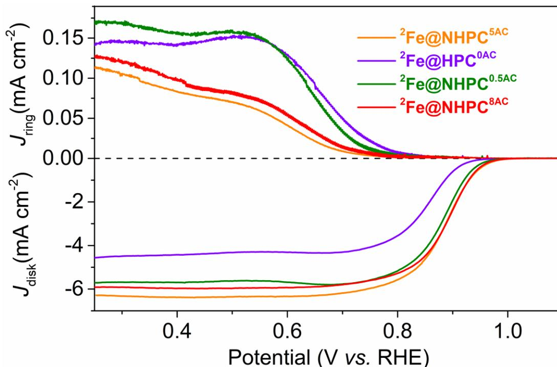
Figure 16. RRDE current-potential curves of samples prepared by different (NH<sub>4</sub>)<sub>2</sub>CO<sub>3</sub> addition at 293 K for ORR in O<sub>2</sub> saturated 0.1 M KOH solution recorded at the Pt-ring potential of 1.2 V (vs. RHE). All ring currents have been measured at an angular rotation rate ( $\omega$ ) of 1600 rpm.
