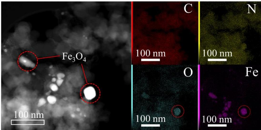
Figure 3. Energy-dispersive-X-ray (EDX) mapping on the  $^{4.5}\text{Fe@NGC/CB}$ .
