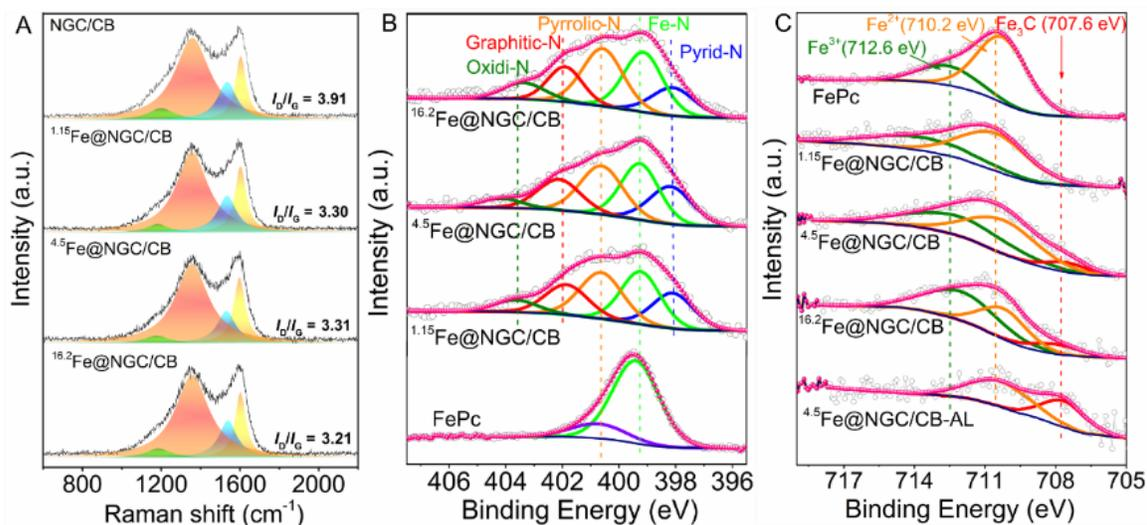
Figure 6. (A) The Raman spectra of samples prepared with different amount of Fe precursor; (B) XPS spectra of high-resolution N 1s core region in the samples containing variably Fe content along with FePc as reference sample at comparison; (C) XPS spectra of high-resolution Fe 2p<sub>3/2</sub> core regions in all concerned samples.
