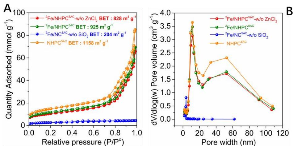
Figure 5. A) N<sub>2</sub> adsorption-desorption isotherm linear plot of <sup>2</sup>Fe/NHPC<sup>5AC</sup>, <sup>2</sup>Fe/NHPC<sup>5AC</sup>-w/o ZnCl<sub>2</sub>, <sup>2</sup>Fe/NC<sup>5AC</sup>-w/o SiO<sub>2</sub>, and NHPC<sup>5AC</sup> recorded at 77 K and respective pore size distribution determined by BJH method using the desorption branch of N<sub>2</sub> isotherm (the data recorded with a pore width from 1.7 nm to 100 nm).
