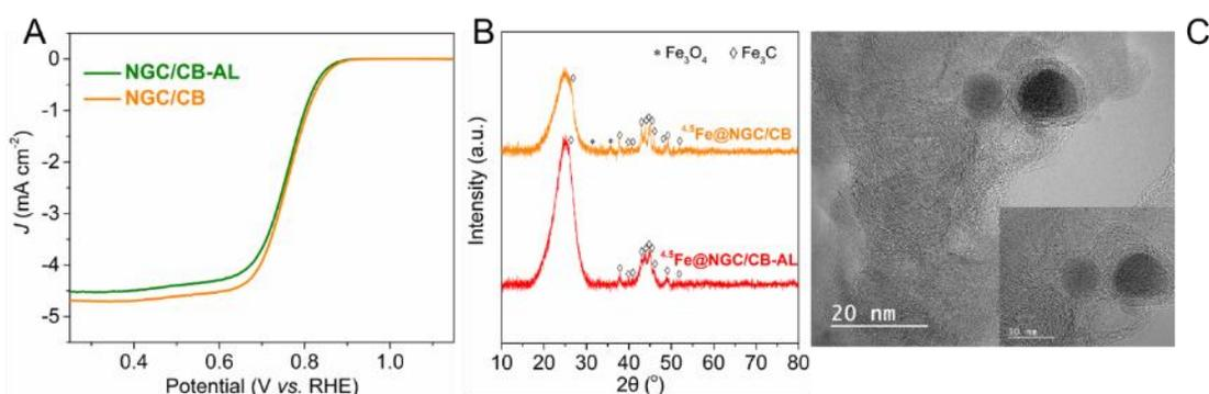
Figure 14. (A) LSVs for NGC/CB and respective acid-leached sample NGC/CB-AL; (B) The XRD patterns of  $^{4.5}\text{Fe}@NGC/\text{CB}$  and respective acid-leached sample  $^{4.5}\text{Fe}@NGC/\text{CB}-\text{AL}$ ; (C) TEM images at different magnification for sample  $^{4.5}\text{Fe}@NGC/\text{CB}-\text{AL}$ .
