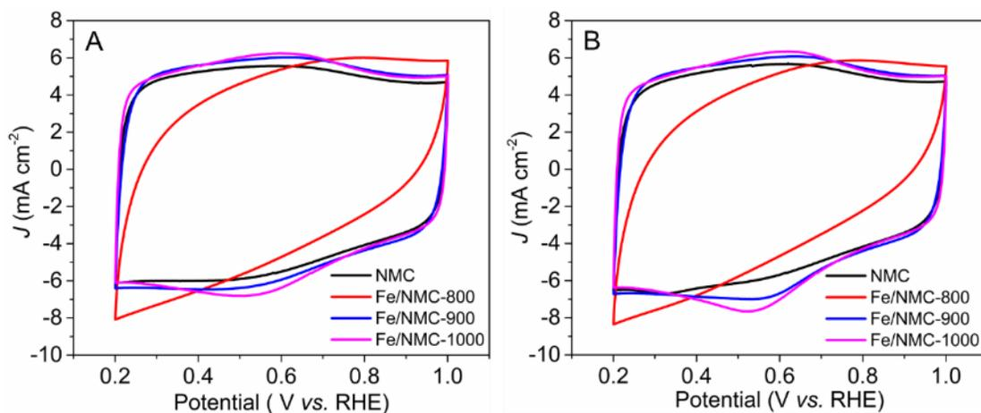
Figure 7. Cyclic voltammetry of as-prepared under N<sub>2</sub>-saturated (A) and O<sub>2</sub>-saturated (B) 0.5 M H<sub>2</sub>SO<sub>4</sub> solution at scan rate of 50 mV s<sup>-1</sup>.
