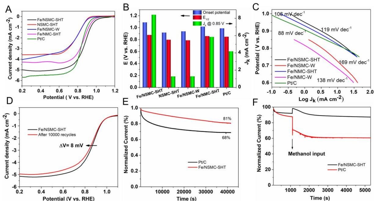
Figure 12. (A) ORR polarization curves, (B) Onset Potential, half-wave potential ( $E_{1/2}$ ) and kinetic current density ( $J_k$ ) for different catalysts, (C) Tafel slop for as-prepared catalysts, (D) Accelerated durability test (ADT) for Fe/NSMC-SHT, (E) CA response for Fe/NSMC-SHT, (F) methanol tolerance test for Fe/NSMC-SHT.
