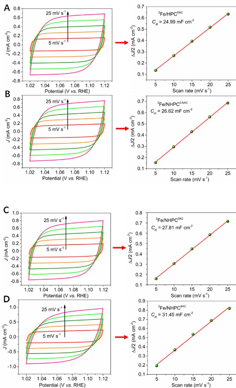
Figure 18. The CV curves in the potential range of 1.02-1.12 V vs. RHE with various scan rates in  $N_2$ -saturated 0.1 M KOH solution and corresponding linear fitting of the capacitive currents vs. scan rates for (A)  $^2Fe/HPC^{0AC}$ ; (B)  $^2Fe/NHPC^{0.5AC}$ ; (C)  $^2Fe/NHPC^{5AC}$ ; (d)  $^2Fe/NHPC^{8AC}$ .
