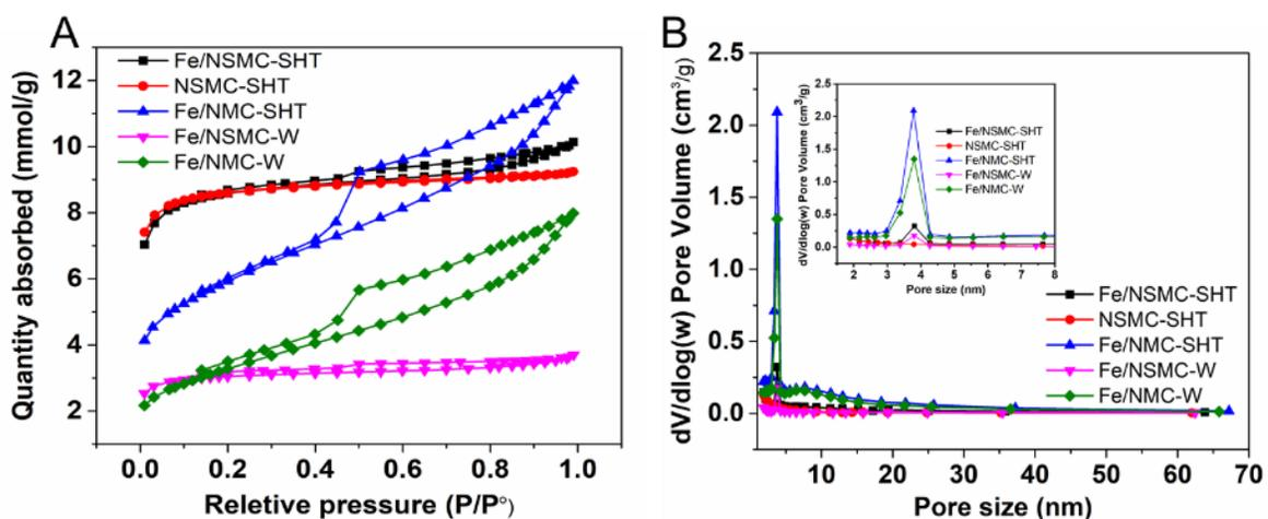
Figure 9. (A)  $N_2$  adsorption-desorption isotherms curves recorded at 77 K, and (B) respective pore size distribution curves with Barrett-Joyner-Halenda (BJH) method based on desorption branches of representative samples.
