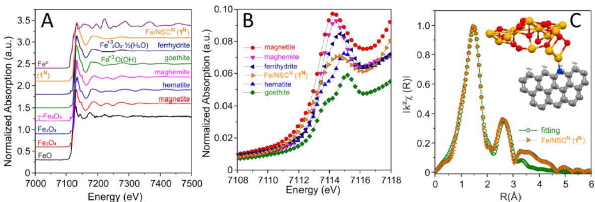
Figure 10. A) Normalized XANES spectra for model catalyst (1<sup>N</sup> is referred to as Fe/NSMC-SHT for the sake of convenience) and more common iron oxide samples or metallic iron. B) Magnification section of Figure 10A dealing with the absorption pre-edge (1s → 3d) resonances. C) k<sup>2</sup> weighted Fourier transform of EXAFS data of model catalyst and related fit. Color codes for the inset: C = gray, H = white, N = blue, Fe = orange, O = red
