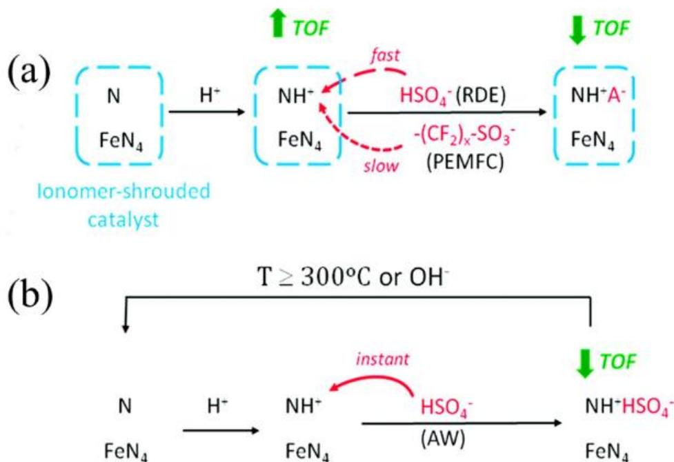
**Figure 9.** Change of the chemical state of protonable N-groups and simultaneous change of the turnover frequency (TOF) for the ORR of FeN<sub>4</sub> catalytic sites when the Fe/N/C catalyst is shrouded by proton-conducting ionomer (a) or directly in contact with an aqueous acidic solution (b). In case (b), the acid-washed catalyst can be reactivated either thermally or chemically. Reproduced from Ref. [106]
