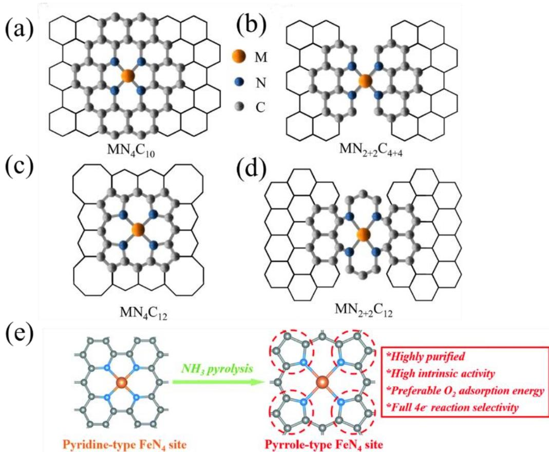
**Figure 13.** Proposed active site structures for Fe-centered moieties. (a) Pyridinic in-plane  $FeN_4C_{10}$  moiety, (b) pyridinic armchair edge  $FeN_{2+2}C_{4+4}$  moiety, (c) porphyrinic in-plane  $FeN_4C_{12}$  moiety, (d) porphyrin zig-zag edge  $FeN_{2+2}C_{12}$  moiety, (e) schematic illustration of preparation of high-purity pyrrolic-type  $FeN_4$  site. Reproduced from Ref. [178, 179]
