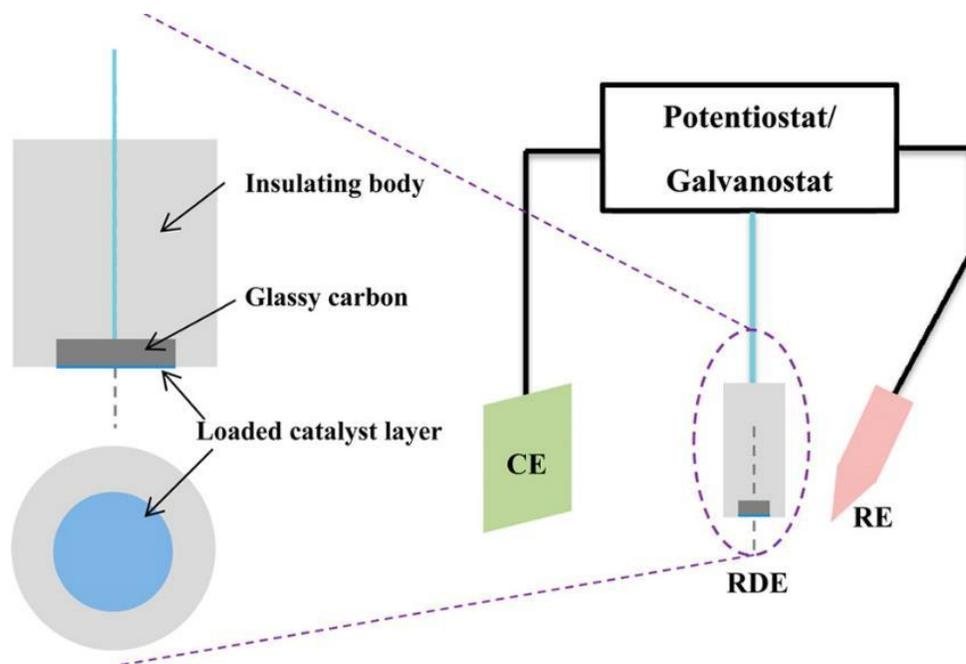
**Figure 4.** Schematic diagram of typical rotating-disk electrode (RDE) testing setup in three-electrode configuration. Reproduced from Ref. [81]
