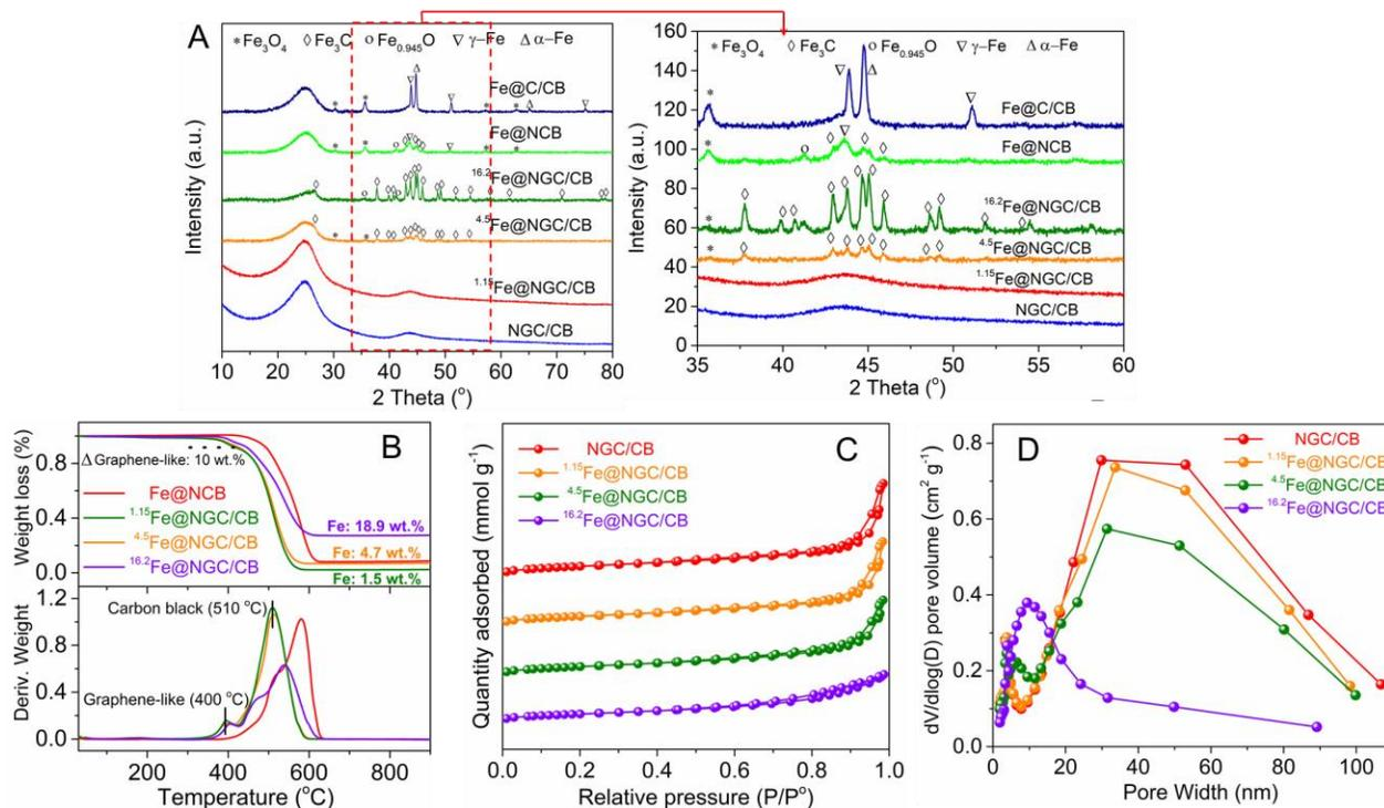
Figure 4. (A) The XRD profiles of all as-prepared catalysts; (B) The TGA (above) and DTG (below) curves of <sup>1.15</sup>Fe@NGC/CB, <sup>4.5</sup>Fe@NGC/CB, <sup>16.2</sup>Fe@NGC/C, and Fe/NCB; (C) N<sub>2</sub> adsorption-desorption isotherm plots of samples with variable Fe addition recorded at 77 K along with (D) the respective pore size distributions (BJH method) based on desorption branch.
