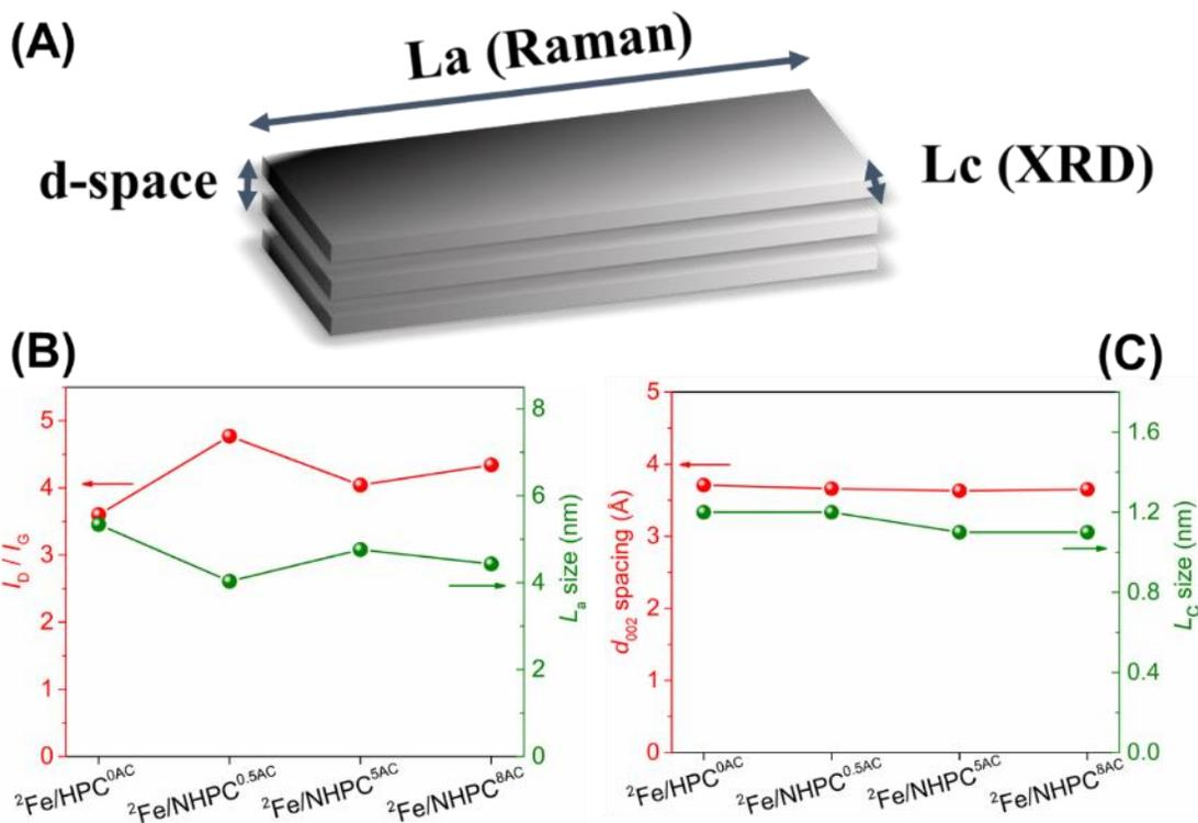
Figure 17. (A) The proposed model of carbon structure; (B)  $I_D/I_G$  values and  $L_a$  sizes obtained from Raman spectra; and (C) the  $d$  spacing values and  $L_c$  sizes from XRD analysis as function of addition amount of  $(\text{NH}_4)_2\text{CO}_3$ .
