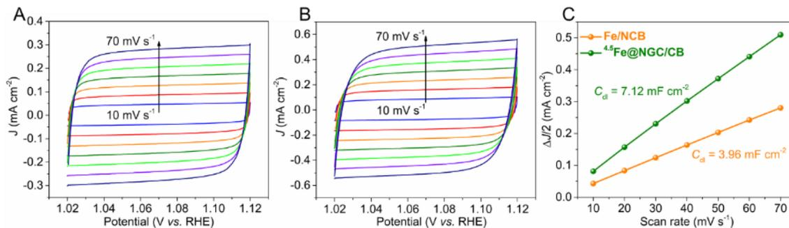
Figure 10. The CV curves of Fe@NCB (A) and  $^{4.5}\text{Fe@NGC/CB}$  (B) in the potential range of 1.02-1.12 V vs. RHE with various scan rates in  $\text{N}_2$ -saturated 0.1 M KOH solution and corresponding linear fitting of the capacitive currents vs. scan rates (C).
