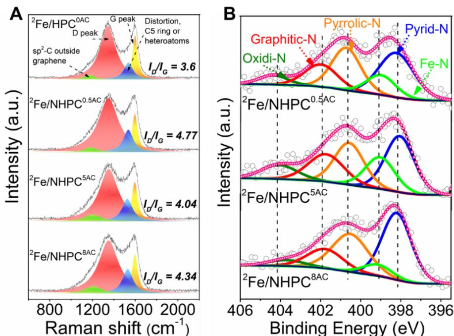
Figure 10. (A) Raman spectra of samples using various amount of (NH<sub>4</sub>)<sub>2</sub>CO<sub>3</sub>; (B) XPS spectra of high-resolution N 1s core region in the N-containing catalysts.
