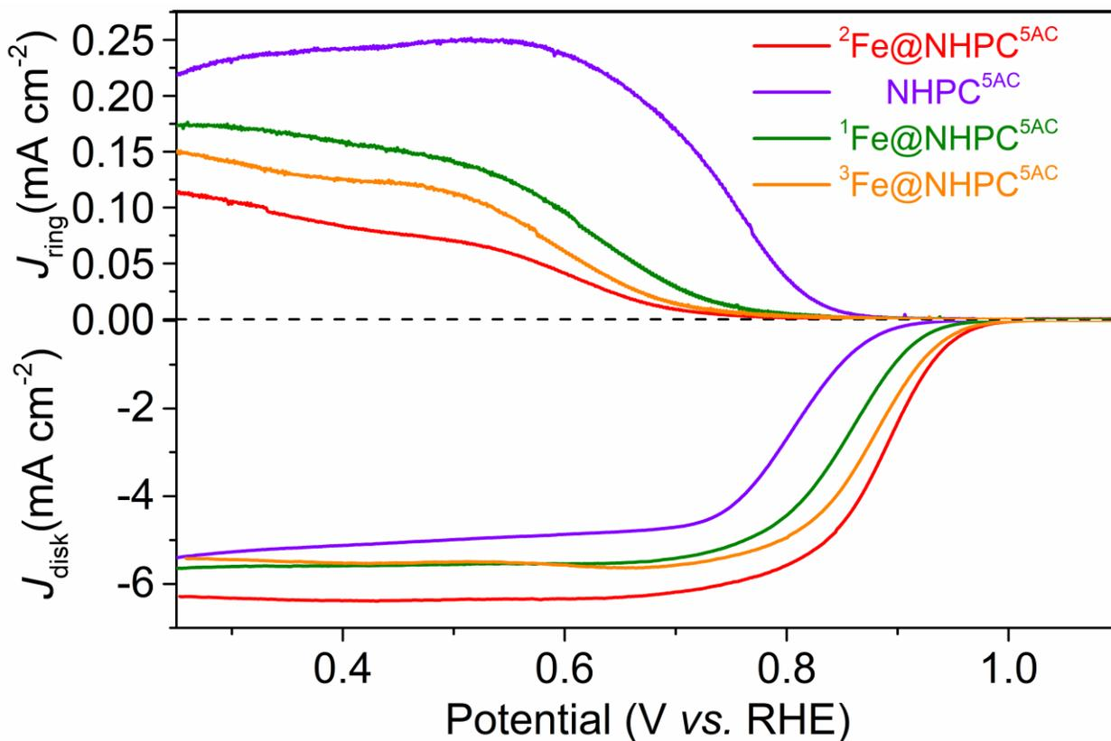
Figure 20. RRDE current-potential curves of samples prepared by different Fe addition at 293 K for ORR in O<sub>2</sub> saturated 0.1 M KOH solution recorded at the Pt-ring potential of 1.2 V (vs. RHE). All ring currents have been measured at an angular rotation rate ( $\omega$ ) of 1600 rpm.
