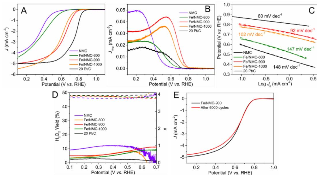
Figure 8. (A) LSVs curves of as-prepared along with commercial Pt/C catalyst at comparison recorded at O<sub>2</sub>-saturated 0.5 M H<sub>2</sub>SO<sub>4</sub> solution at a scan rate of 10 mV s<sup>-1</sup> with rotation speed of 1600 rpm; (B) Respective ring current density curves; (C) Tafel slope extracted by LSVs curves in the disk electrode; (D) H<sub>2</sub>O<sub>2</sub> yield and electron transfer number derived from RRDE measurement; (E) The durability test for Fe/NMC-900.
