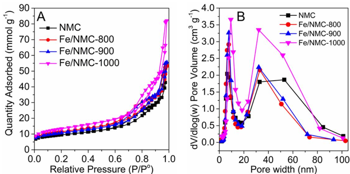
Figure 4. (A)  $\text{N}_2$  adsorption/desorption isotherm plots for as-prepared catalysts recorded at 77 K; and (B) respective pore size distribution curves using desorption branch of isotherms for all samples (BJH method, the data recorded with a pore width from 1.7 nm to 100 nm).
