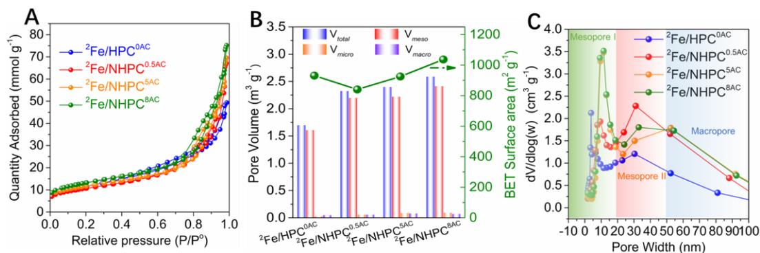
Figure 4. (A)  $\text{N}_2$  adsorption-desorption isotherm plots for samples with different amount of  $(\text{NH}_4)_2\text{CO}_3$  recorded at 77 K; (B) The correlation plots of specific surface area (SSA) and pore volume as function of addition of  $(\text{NH}_4)_2\text{CO}_3$ ; (C) The respective pore size distribution using the desorption branch of  $\text{N}_2$  isotherms (BJH method, the data recorded with a pore width from 1.7 nm to 100 nm).
