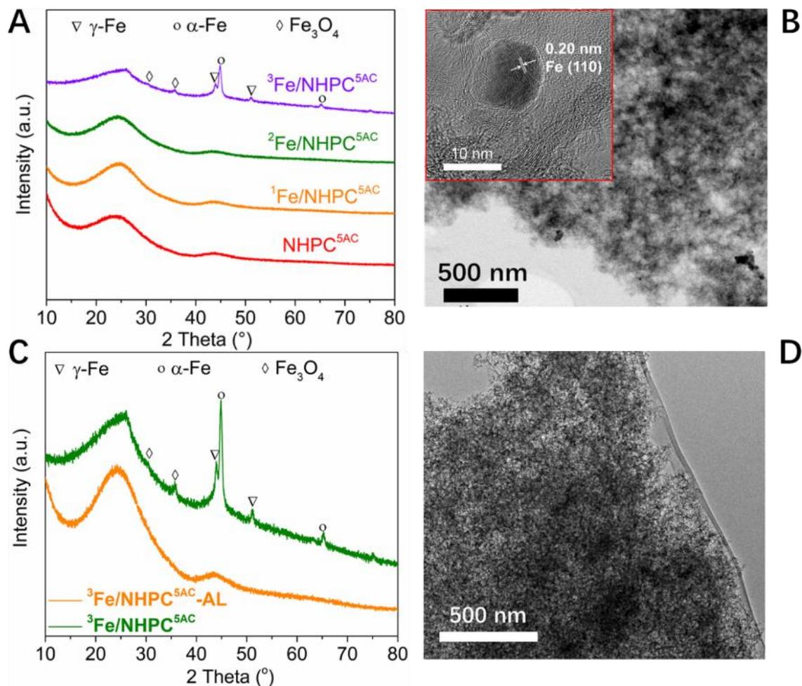
Figure 21. (A) XRD patterns of as-obtained catalysts using different amount of Fe precursor; (B) TEM image of  $^3\text{Fe}/\text{NHPC}^{5\text{AC}}$  (HRTEM shown in the inset); (C) XRD patterns of  $^3\text{Fe}/\text{NHPC}^{5\text{AC}}$  and  $^3\text{Fe}/\text{NHPC}^{5\text{AC}}\text{-AL}$ ; (D) TEM image of  $^3\text{Fe}/\text{NHPC}^{5\text{AC}}\text{-AL}$ .
