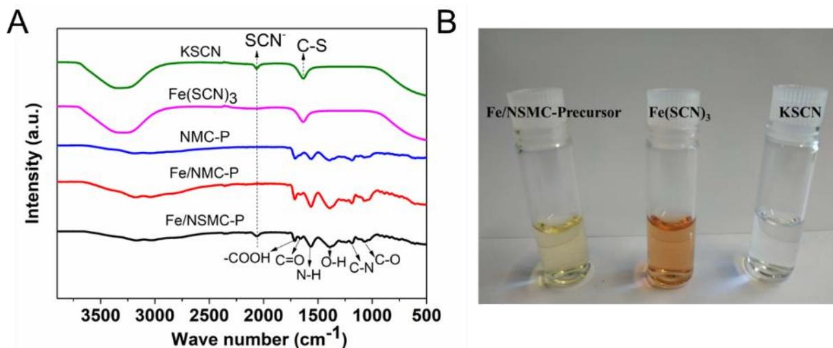
Figure 1 (A) ATR-FTIR spectra of Fe/NSMC, Fe/NMC and NMC precursor gel after  $110\text{ }^\circ\text{C}$  drying as well as KSCN and  $\text{Fe}(\text{SCN})_3$  aqueous solution; (B) Digital photos of Fe/NSMC precursor,  $\text{Fe}(\text{SCN})_3$  and KSCN aqueous solution.
