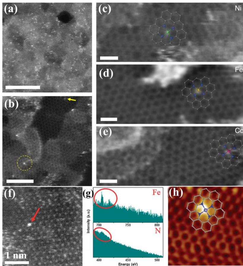
**Figure 12.** (a-e) Atomic structure characterizations of M-NHGFs by annular dark-field STEM. (f) High-angle annular dark-field scanning transmission electron microscopy (HAADF-STEM) image. (g) the electron energy loss spectroscopy (EELS) atomic spectra of elemental Fe and N from the bright dots. (h) Low temperature scanning tunneling microscopy (LS-STM) image of FeN<sub>4</sub>/GN. Reproduced from Ref. [166, 167]
