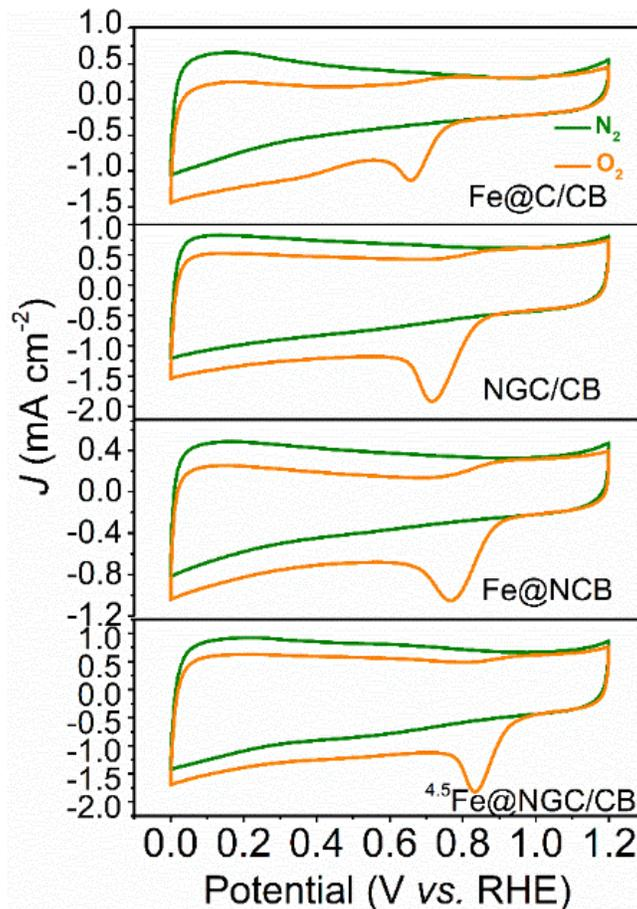
Figure 8. The CV curves of control samples at potential range of 0 - 1.2 V vs. RHE with a scan rate of  $50 \text{ mV s}^{-1}$  under  $\text{N}_2$  and  $\text{O}_2$ - saturated 0.1 M KOH solution, respectively.
