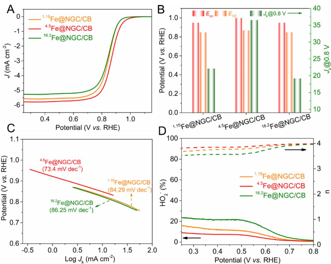
Figure 12. (A) Steady-state polarization curves of samples produced by the use of different Fe precursor and (B) respective electrochemical parameter ( $E_{on}$ ,  $E_{1/2}$ , kinetic current density,  $J_k@0.8$  V); (C) Tafel plots for samples prepared by variably addition of Fe; (D) The  $H_2O_2$  yield and electron transfer number for samples with different Fe loadings derived from rotation disk-ring
