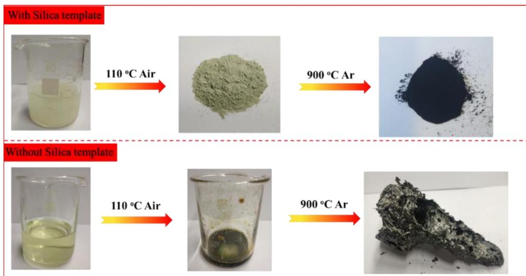
Figure 2. The digital picture of synthetic procedure of model catalyst  ${}^2\text{Fe}/\text{NHPC}^{5\text{AC}}$  (above), and control sample  ${}^2\text{Fe}/\text{NC}^{5\text{AC}}\text{-w/o SiO}_2$  (below).
