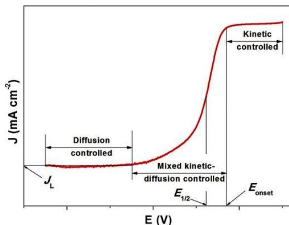
**Figure 5.** Typical ORR polarization curve. Reproduced from Ref. [82]
