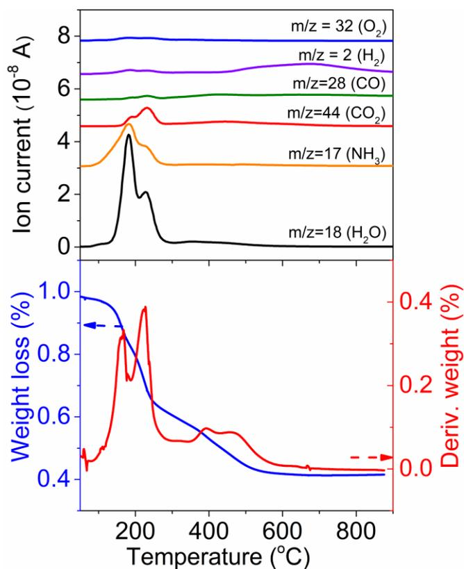
Figure 3. TPD-MS (above) and corresponding TGA plots (below) of precursor powder of <sup>2</sup>Fe/NHPC<sup>5AC</sup> after a drying step at 110 °C.
