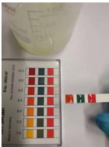
Figure 1. The digital picture of pH value for precursor sol solution of model catalyst.
