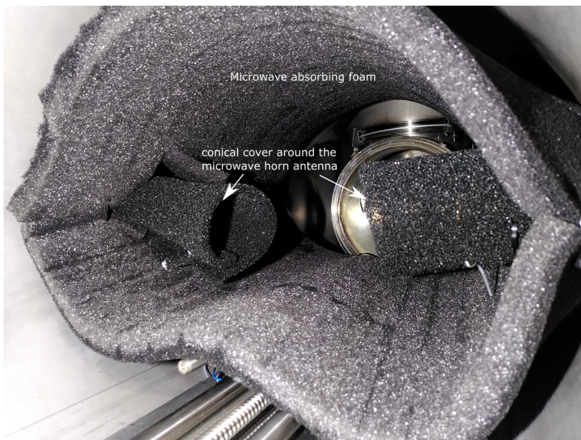
Figure 2.13: Picture of the microwave absorbing form layout inside the vacuum chamber.
