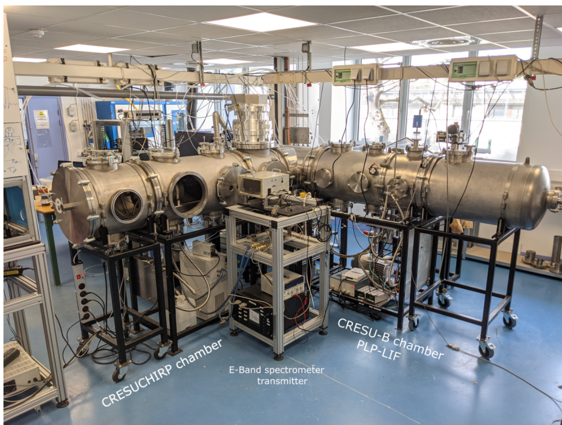
Figure 2.6: Picture of the two CRESU chambers on the left the CRESUCHIRP apparatus and on the right the PLP-LIF apparatus.
