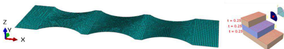
(b) Thin shell elements of CFRP skin.
