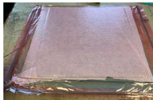
(b) Sealed vacuum bag of CFRP laminates.
