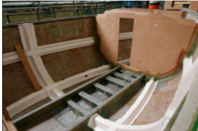
Fig. 1-6. GFRP-balsa sandwich applied in the ship hull [38].
