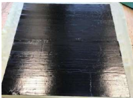
(a) Lay-up of CFRP prepreg plies.
