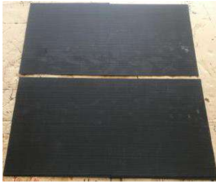
(a) Cured CFRP laminates.
