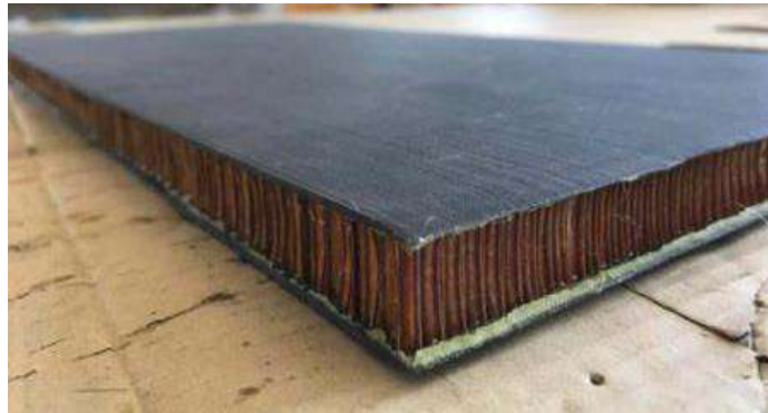
(c) Cured CFRP-honeycomb sandwich.
