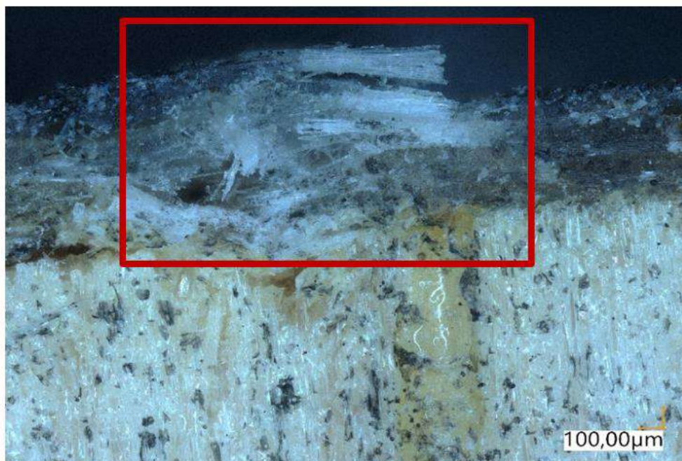
Fig. C. Zoom of skin damages of Dry 1.
