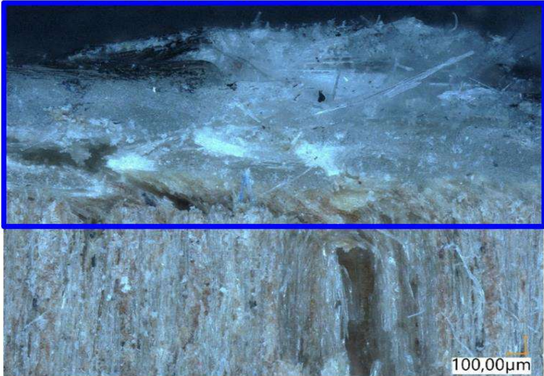
Fig. B. Zoom of skin damages of 120% MC specimen Wet 5.
