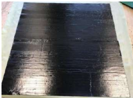
(a) Lay-up of CFRP prepreg plies.
