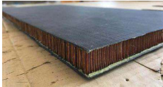
(c) Cured CFRP-honeycomb sandwich.
