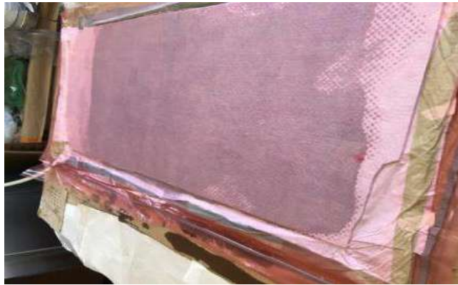
(c) Sealed vacuum bag of GFRP-balsa sandwich.
