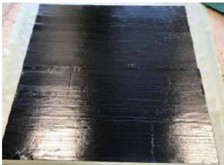
(a) Lay-up of CFRP prepreg plies.
