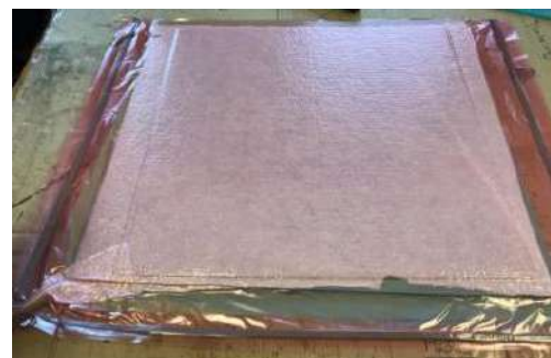
(b) Sealed vacuum bag of CFRP laminates.
