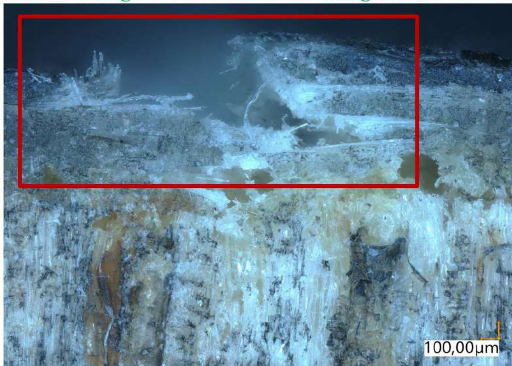
Fig. C. Zoom of skin damages of 50% MC specimen Wet 2.
