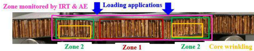
(e) The real damage surfaces of the honeycomb core after the test.
