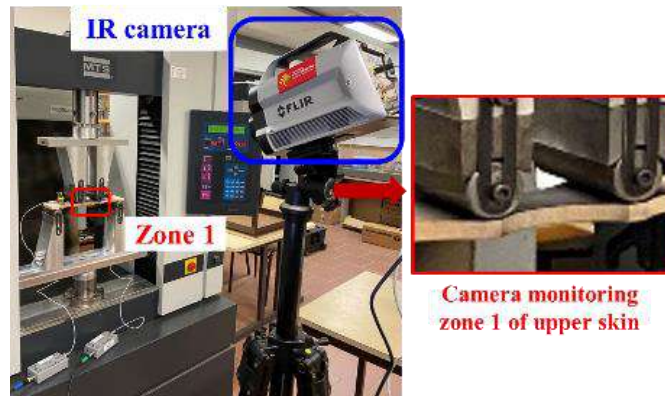
(b) IR camera setup.
