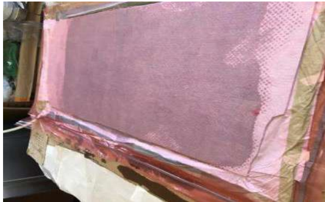
(c) Sealed vacuum bag of GFRP-balsa sandwich.
