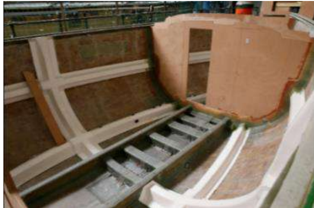
Fig. 1-6. GFRP-balsa sandwich applied in the ship hull [38].
