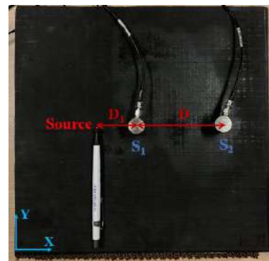
(b) CFRP-honeycomb sandwich panel
