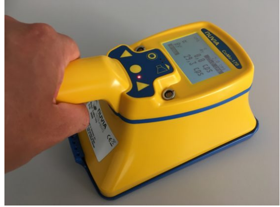
Figure 1.2: Two commercial devices for \alpha/\beta particle detection: the SaphyRAD A-B 170 probe from Bertin Technologies (on the left) and the CoMo 170 from NUVIA Tech Instruments (on the right).
