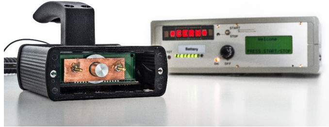
Figure 1.4: On the left, the active probe of one of the first prototypes of the B-RAD without the front cover to show the LaBr 3 crystal; on the right, the control unit.
