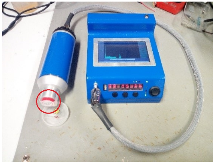
Figure 2.28: Measurement of a ^{137}\text{Cs} source's contact dose rate with the B-RAD. The source is placed in contact with the probe (red circle).
