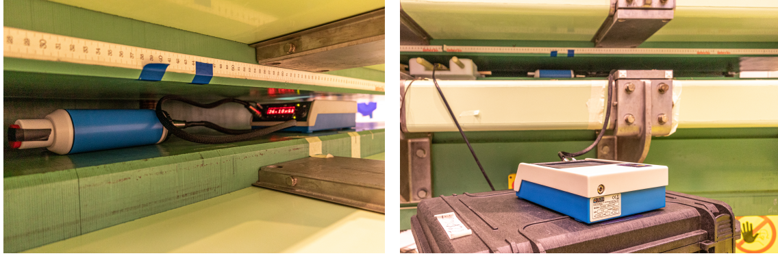
Figure 2.5: Two different working conditions of the B-RAD inside the dipole. On the left, both probe and control unit are inside the dipole magnet and on the right, the probe is inside the dipole while the control unit remains outside.
