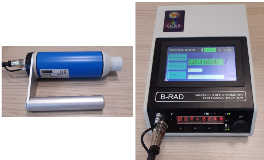
Figure 2.2: On the left, the probe of the latest version of the B-RAD; on the right, the control unit of the same version.
