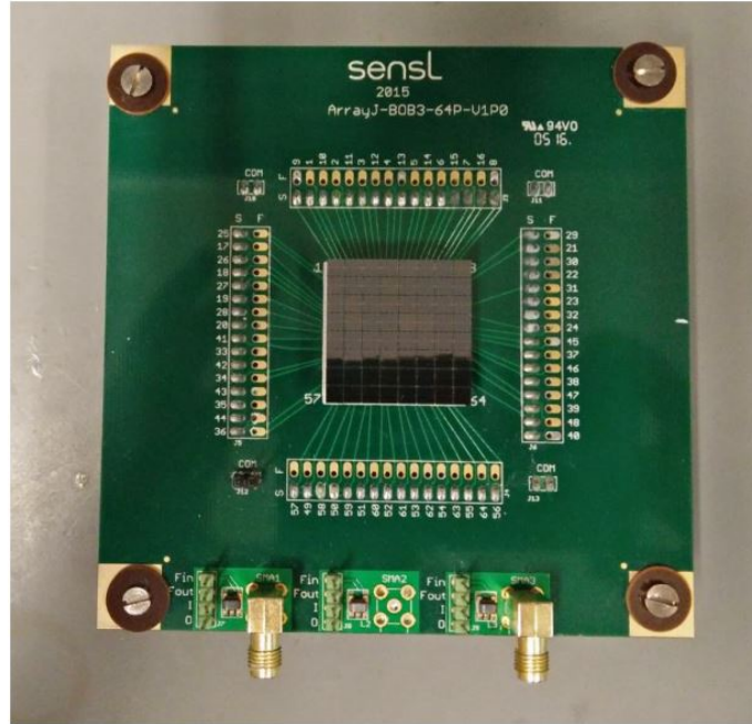
Figure 3.27: The SiPM Array J-30035-64P and the ArrayJ-BOB3-64-V1P0 breakout board used to measure the variation of the breakdown voltage with temperature.
