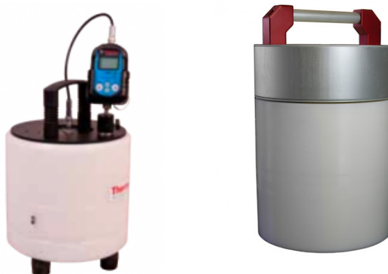
Figure 1.3: Two commercial neutron rem counters: the FHT 762 Wendi-2 from Thermo Fischer Scientific (on the left) and the Lupin BF3-NP from ELSE NUCLEAR (on the right).
