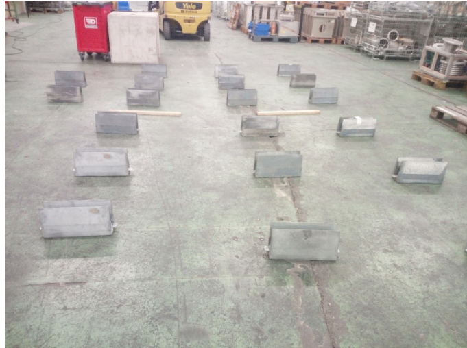
Figure 2.24: The twenty permanent magnets measured with the B-RAD at ISR7.
