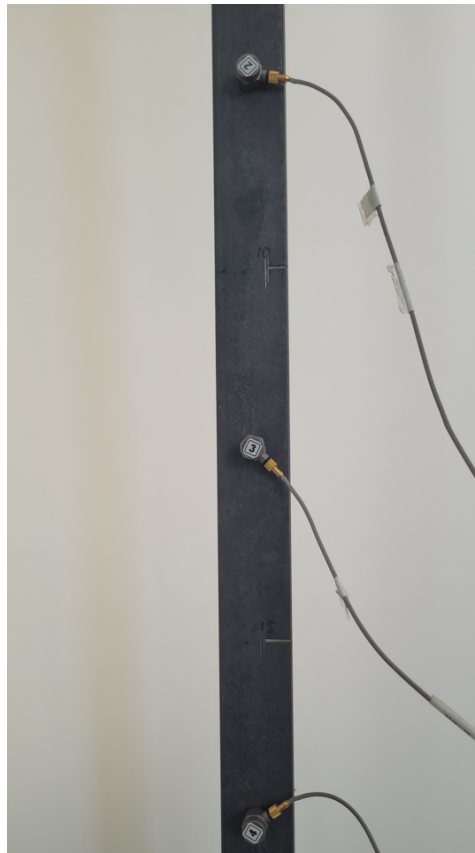
Fig. 9. Experimental setup for the cantilever beam
