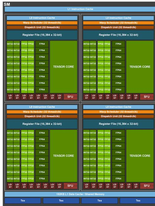
Figure 1.16: The architecture of an Ampere Streaming Multiprocessor.
