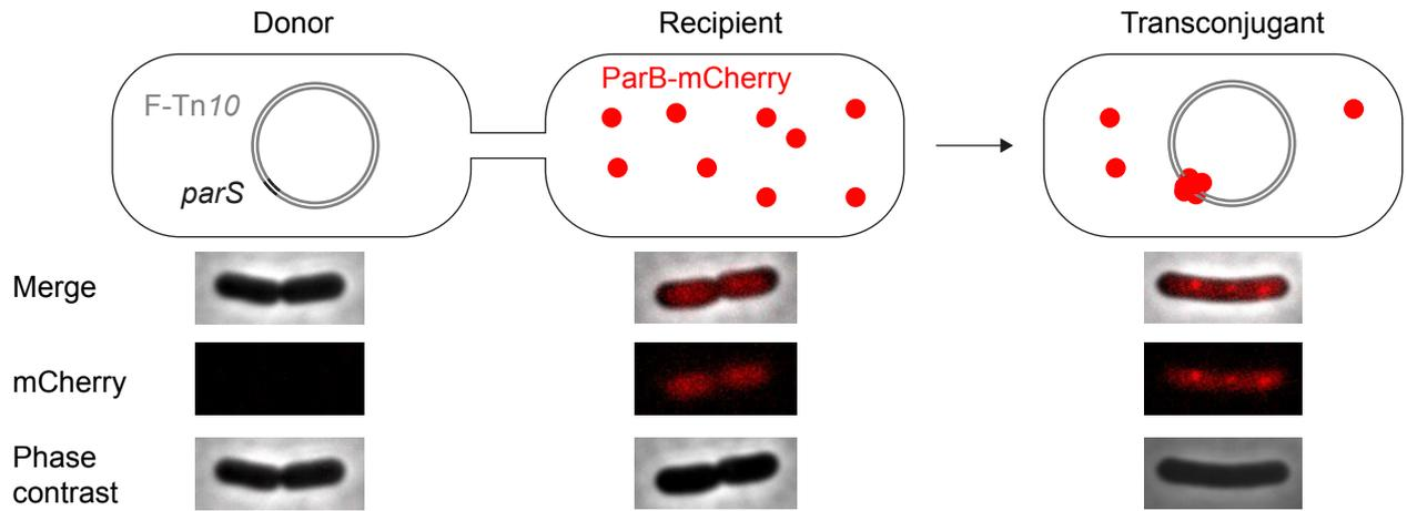
Figure R11 : Transfer visualization system
