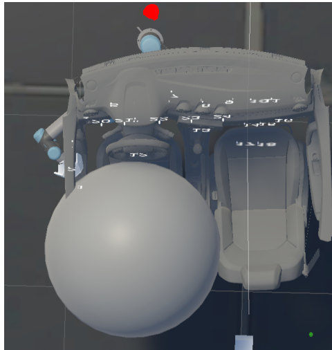
Figure 5.4 – In the definition of the robot motion to joint the ROI, the sphere that represents the user occupancy zone is avoided.
