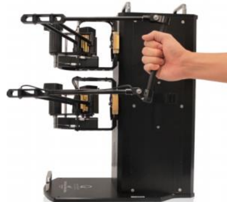
(d) HD2 High Definition Haptic Device from Quanser, Canada.[107]
