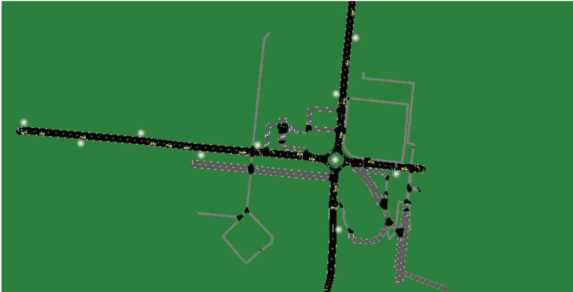
Figure 5.3: SUMO : map of the considered region (the white points indicate the positions of the RSUs)
