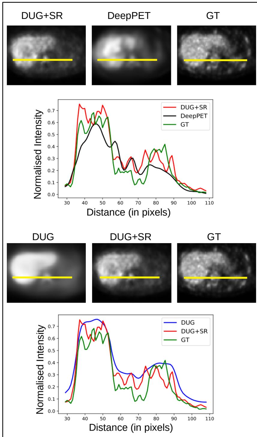
FIGURE 4.13: Intensity Profile across the image (highlighted by a yellow line) for a PET image prediction by DUG, DUG+SR and DeepPET compared with the GT
