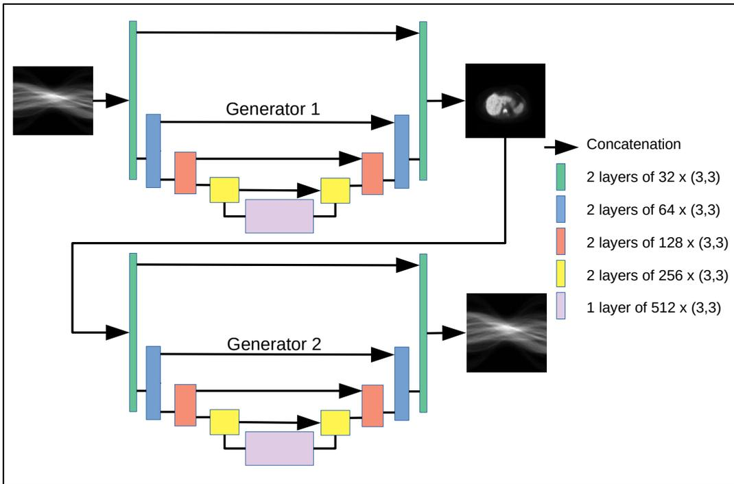
FIGURE 4.3: Representation of the DUG, the image reconstruction block. This network was trained on denoised sinograms which were the outputs of the previous segment.
