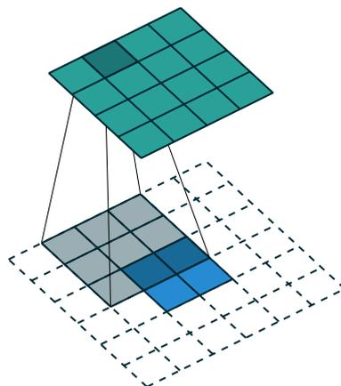
FIGURE 2.7: Transposed convolution over a  $2 \times 2$  input to get a  $4 \times 4$  output. (Dumoulin and Visin, 2016)
