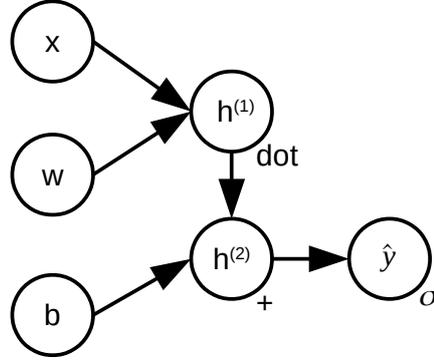
FIGURE 2.2: Computational graph with one hidden layer. The nodes in the first layer store the input  $x$ , weight  $w$  and the bias  $b$ . The second layer contains the hidden layer with 2 units each with the corresponding operation written below. The final layer is the output layer denoted by  $\hat{y} = \sigma(wx + b)$ , where  $\sigma$  is the sigmoid function defined earlier.
