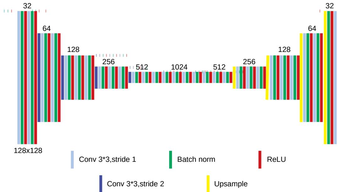
FIGURE 4.8: Representation of DeepPET. The number of filters in each convolutional layer is labeled on top of each block.
