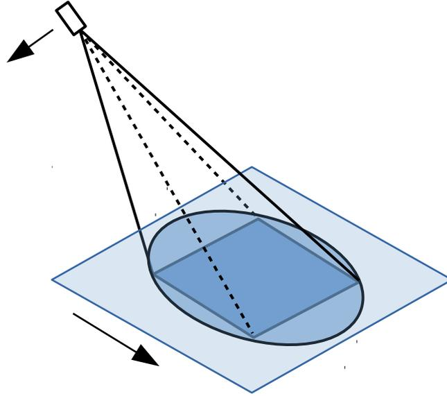
FIGURE 1.5: Cone-beam geometry: the source rotates around the patient while the bed is translated creating a helical scan.
