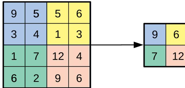
FIGURE 2.5: Max pooling with  $2 \times 2$  filter and stride 1
