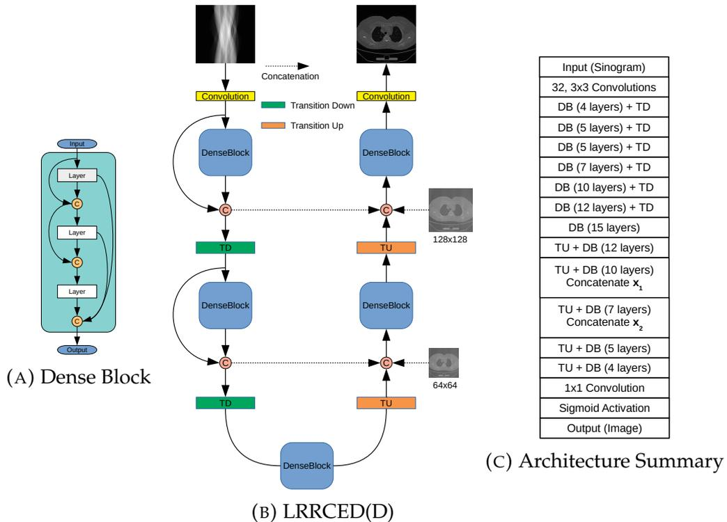
FIGURE 5.2: Different components of LRRCED(D): (a) Representation of a dense block with three layers. (b) LRRCED(D): Fully convolutional dense network with  $x_1$  at  $64 \times 64$  and  $x_2$  at  $128 \times 128$ . (c) Complete architecture summary
