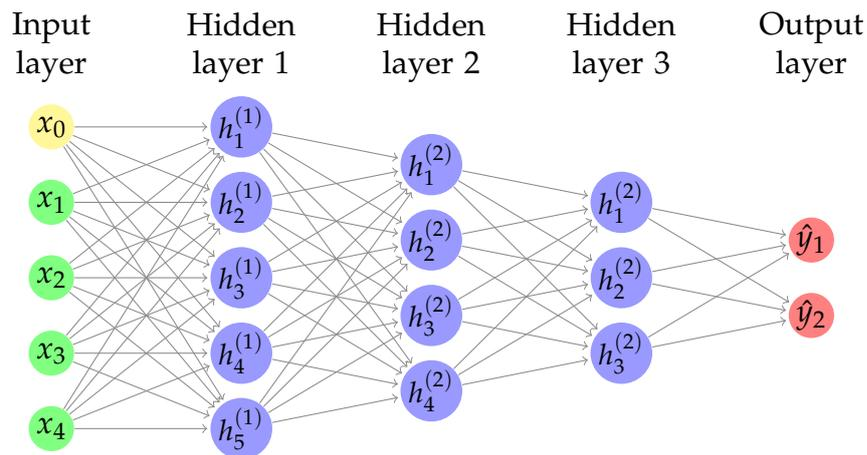
FIGURE 2.1: Depiction of a neural network with an input layer, three hidden layers and an output layer
