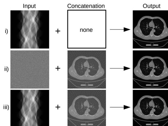
FIGURE 5.16: Schematic representation of configurations used in the ablation study: (i) true sinogram and the reconstructed image only (no low-resolution concatenations); (ii) randomly distributed Gaussian noise sinogram, low-resolution concatenations and the reconstructed images; (iii) true sinogram, low-resolution concatenations and the reconstructed images.
