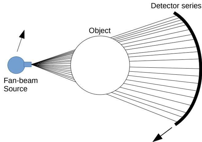
FIGURE 1.4: Fan-beam geometry: the source and the detector rotate around the object
