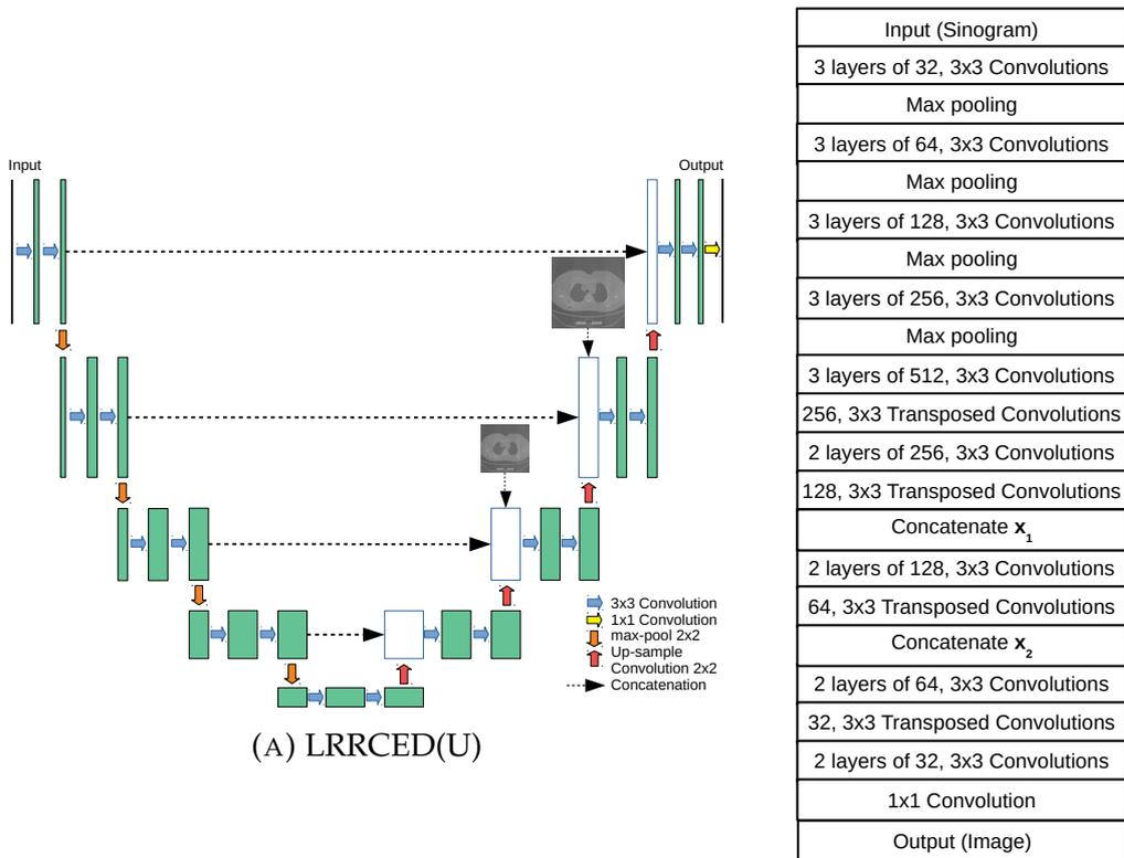
FIGURE 5.3: Different components of LRRCED(U): (a) LRRCED(U): U-Net with  $x_1$  at  $64 \times 64$  and  $x_2$  at  $128 \times 128$ . (b) Complete architecture summary.
