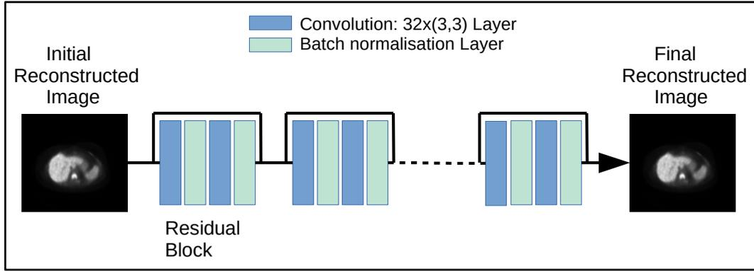
FIGURE 4.4: Representation of the super resolution block. It consists of 8 residual blocks with Convolution, Batch normalization and PReLU.
