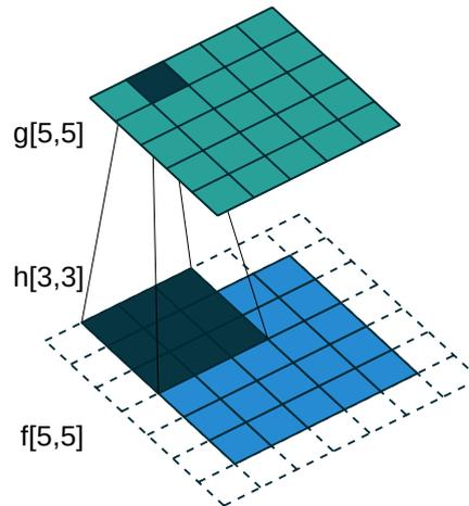
FIGURE 2.3: Convolution of an input image of dimensions  $5 \times 5$  with a filter of dimensions  $3 \times 3$ . (Dumoulin and Visin, 2016)
