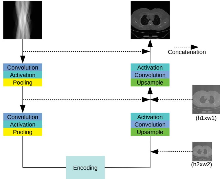
FIGURE 5.1: General representation of an encoder-decoder architecture with fully convolutional layers and the proposed FBP concatenations ( $x_1$  and  $x_2$ ) at two different resolutions  $h_1 \times w_1$  and  $h_2 \times w_2$
