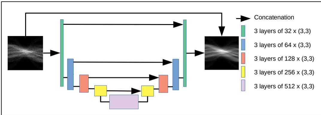
FIGURE 4.2: Representation of the denoising network. The inputs to the network were 2-D grayscale slices with resolution  $128 \times 128$  and the outputs were denoised sinograms.
