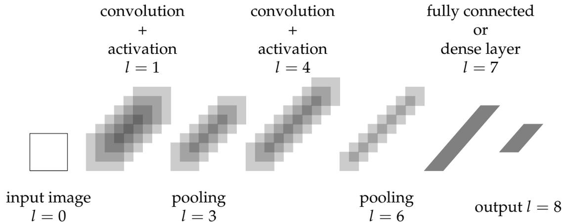
FIGURE 2.6: Architecture of a typical CNN. This representation was first proposed by LeCun and Bengio, 1995.
