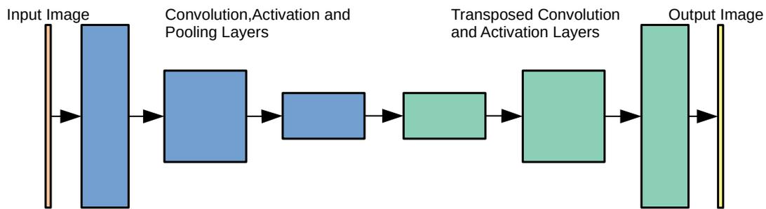
FIGURE 2.8: CNN for image to image translation tasks. This example has an identical structure in convolution path and the transposed convolution path.
