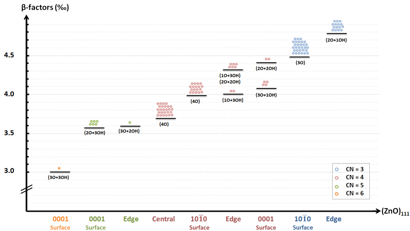
Figure 3.9 Calculated Zn \beta -factors (‰) for (\text{ZnO})_{111} nanoparticle as a function of the position of Zn atoms. Zn atoms are six-fold coordinated (orange), five-fold coordinated
