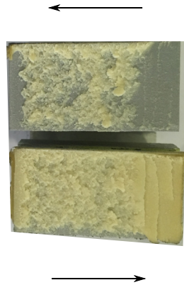
Figure 3.18: Failure surfaces of Arcan specimens bonded with SAF MIB 30 2. Quasi-static test until failure. Arrows designate the direction of each adherend.
