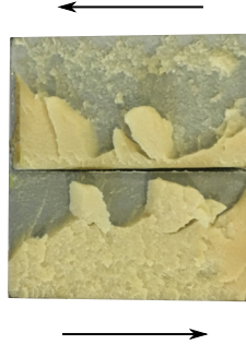
Figure 3.17: Failure surfaces of Arcan specimens bonded with SAF MIB 30 1. Quasi-static test until failure. Arrows designate the direction of each adherend.
