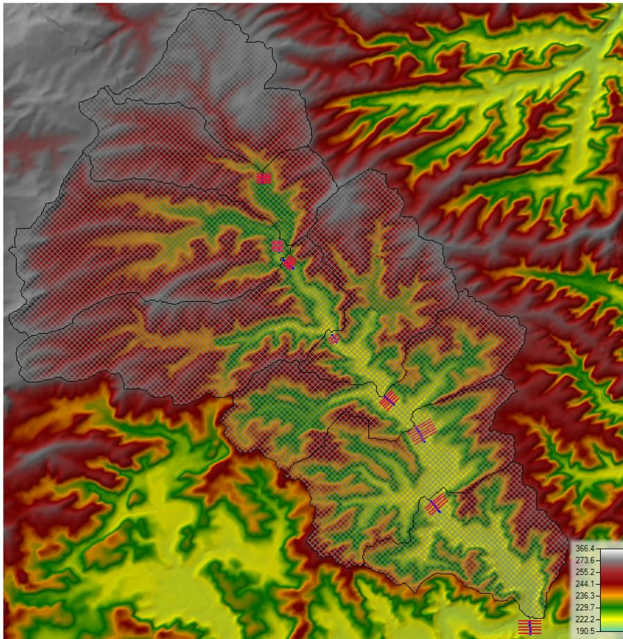
**Figure 5.4:** HEC-RAS model setup of the Moderbach in 8 sub-basins. Each sub-basin (2d flow area) is coupled to a 1D model (river in blue and cross sections in red).
