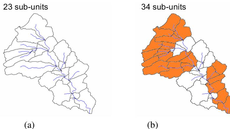
**Figure 3.8:** (a): Partition with the confluence method, (b): Partition with the reach length method (Bassins filled in orange correspond to the additional partitions generated by considering a reach length of 2 km).
