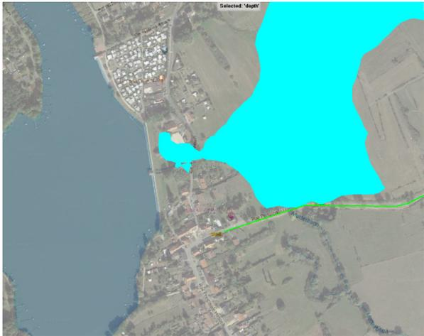
**Figure C.5:** HEC-RAS simulation using the initial DEM.
