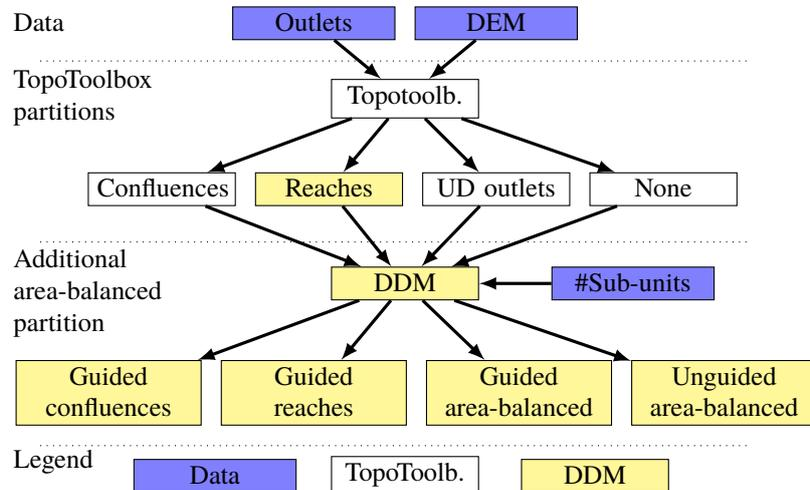
Figure 3.14: Drainage basin partitioning method workflow.
