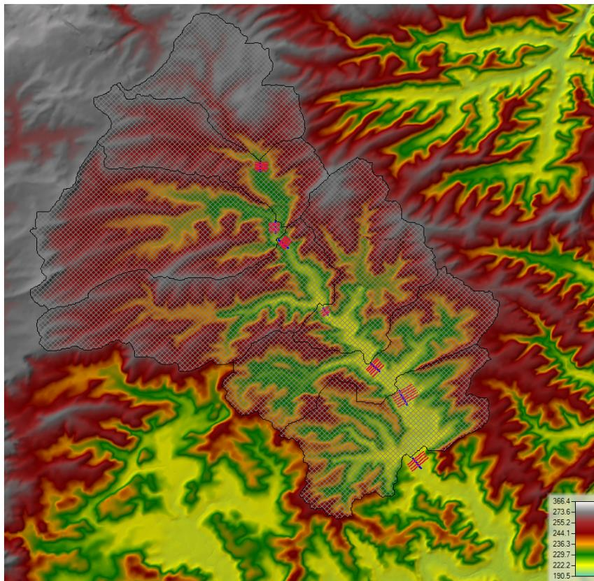
**Figure 5.28:** Computational domain for the precipitation scenario decomposing the Moderbach in 7 sub-basins where each sub-basin (2d flow area) is coupled to a 1D model (river in blue and cross sections in red).
