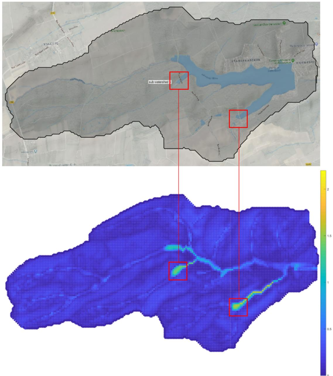
**Figure 4.7:** Visualization of water depth on the sub-basin of Diefenbach with a focus on high water level cells.
