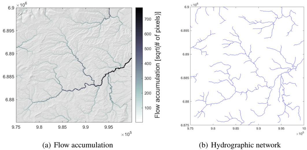
**Figure 3.4:** Deriving drainage basin characteristics (Coordinate system: Lambert-93).
