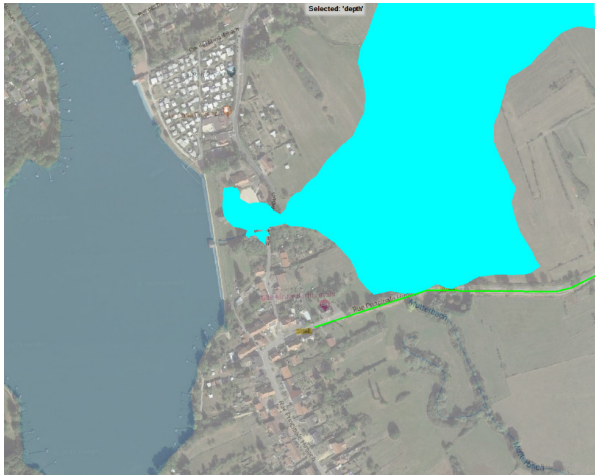
Figure C.5: HEC-RAS simulation using the initial DEM.
