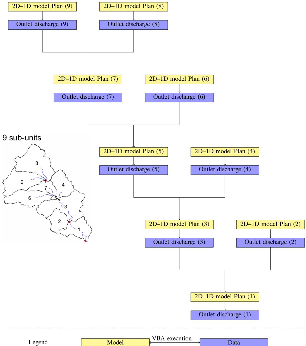
**Figure 5.6:** VBA algorithm organizing the sequential simulation of the 9 sub-basins of the Moderbach generated with the confluence method.
