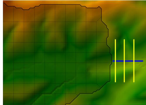
Figure 5.3: 2D-1D model in HEC-RAS (showing the stream in blue and the cross-section in yellow).
