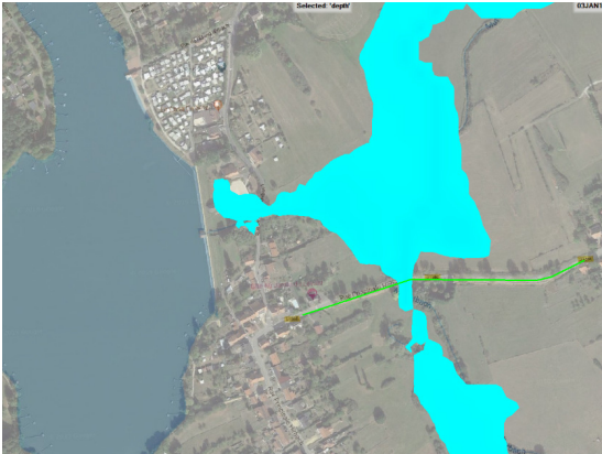
Figure C.7: HEC-RAS simulation with the breached DEM.
