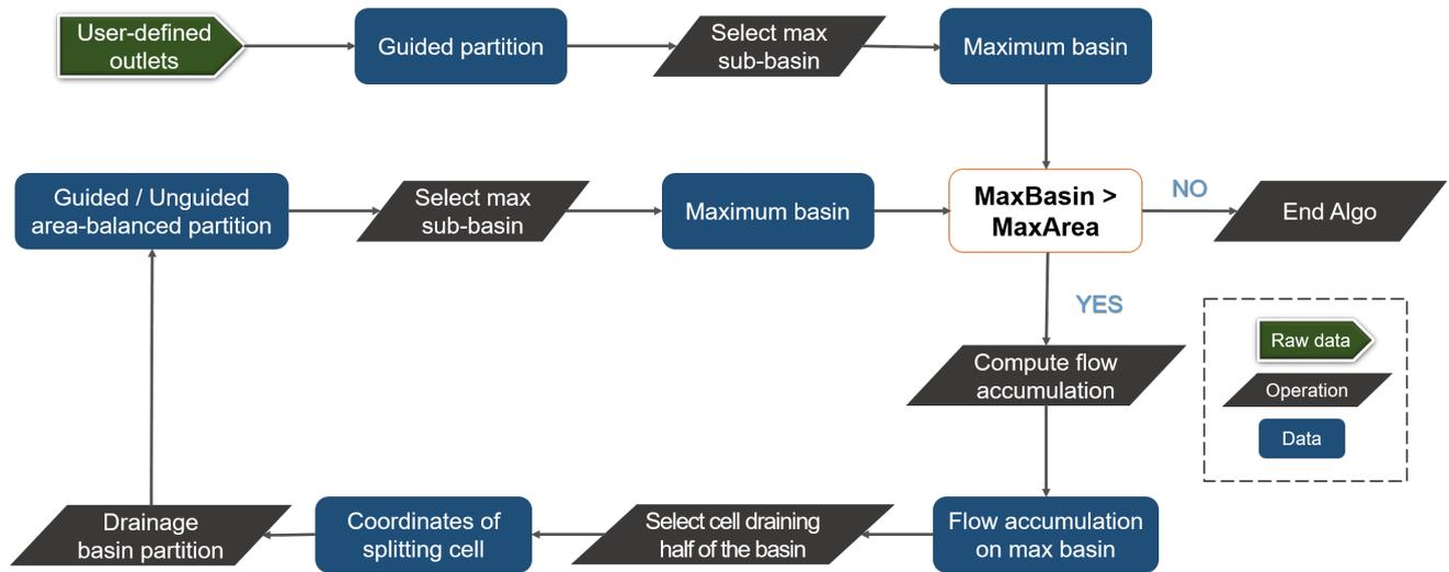
Figure 3.10: Area-balanced drainage basin partitioning method workflow.
