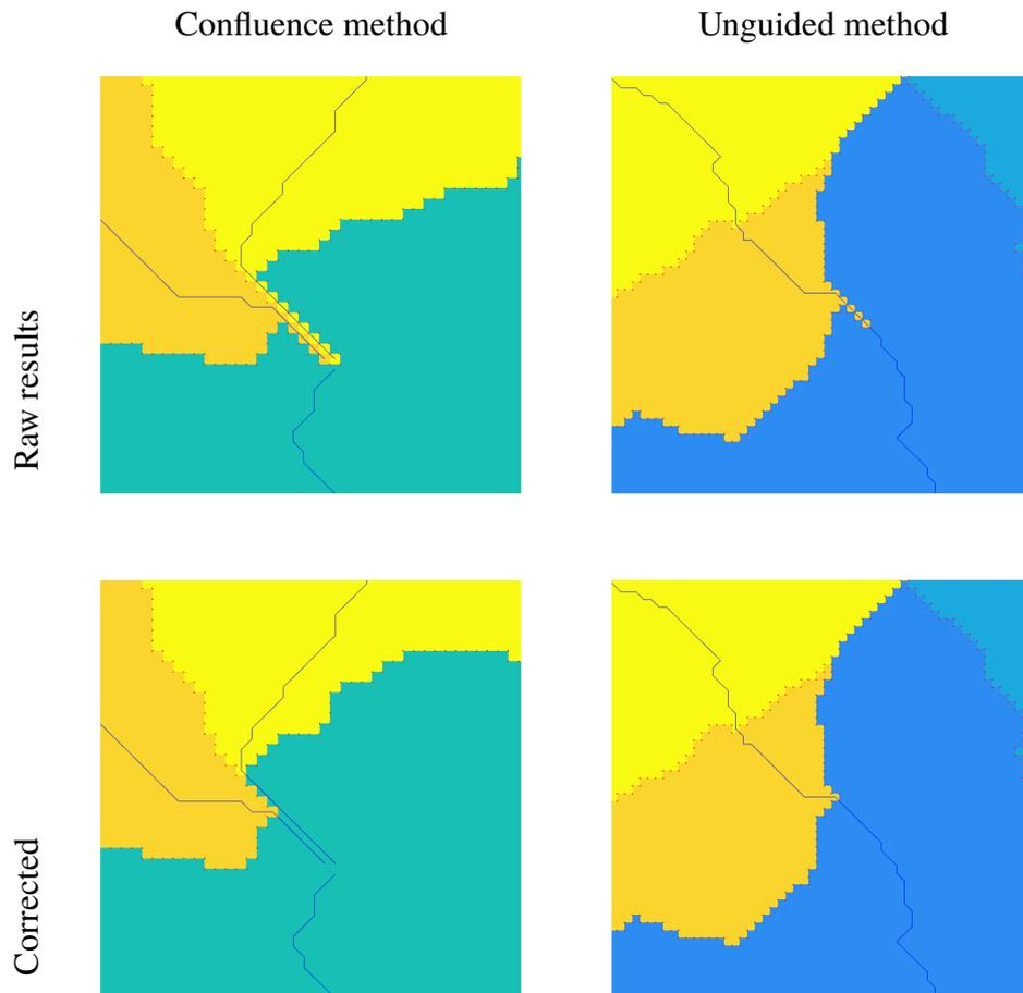
**Figure 3.16:** Isolated cells near to the outlet. Left: Decomposition at the confluences. Right: Unguided area-balanced partition.
