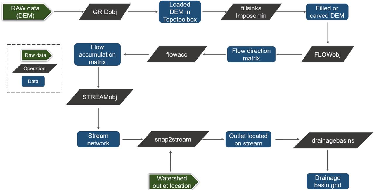
Figure 3.2: Basin delineation process using the Topotoolbox.
