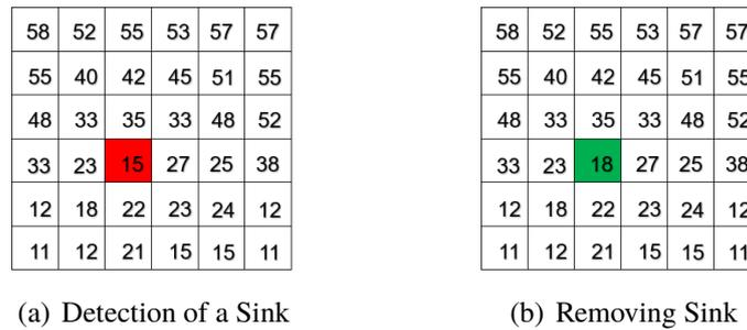
**Figure 4.11:** Detection and correction of a sink.
