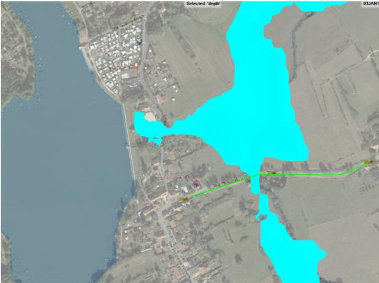
**Figure C.7:** HEC-RAS simulation with the breached DEM.
