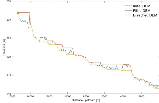
Figure C.1: Stream network longitudinal profile of different DEMs.
