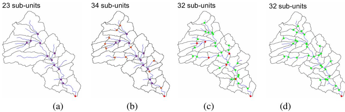
**Figure 3.15:** Comparison of area-balance of different basin partitioning methods a: Partition at confluences (magenta dots), b: Additional partition with respect to a reach length of 2 km (orange dots), c: Guided (red dots) area balanced (green dots) partition, d: Unguided area balanced partition (green dots).
