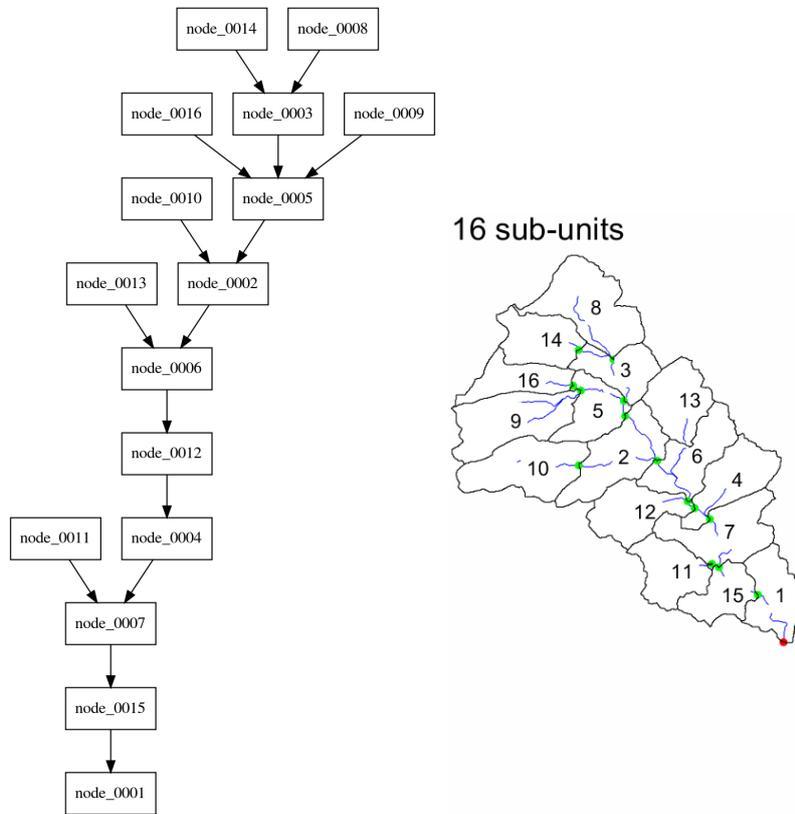
**Figure 4.24:** An illustration of the hierarchical communication relationship for the 16 sub-basins of the Moderbach supported by ORWL.
