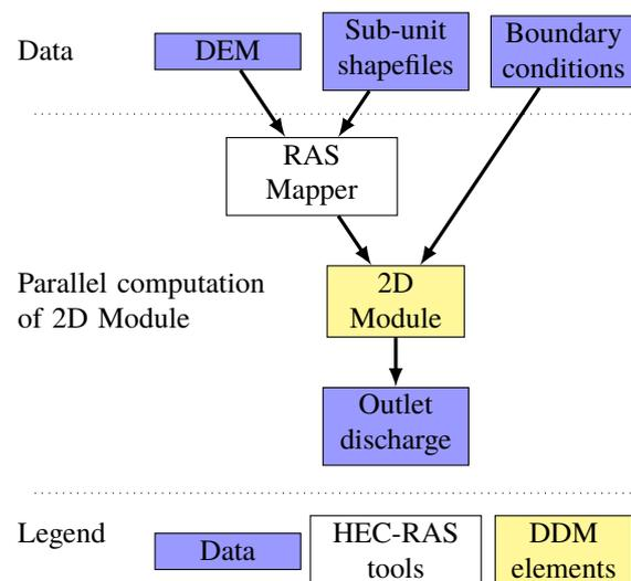
**Figure 4.1:** HEC-RAS workflow for a unique 2D rain-on-grid simulation.
