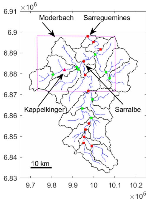
**Figure 5.39:** Area balanced partition of the French Saar catchment into 20 sub-basins at gauging stations (red dots) and additional points (green dots). The magenta box delineates the observation area.
