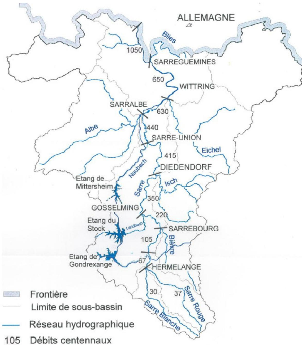
Figure 1.10: The hydrographic network of the Saar watershed (PPRI, 1998).
