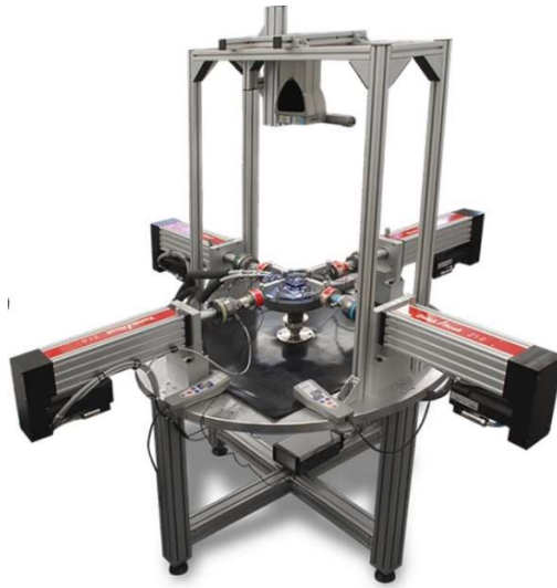
Figure 81. Zwick biaxial tensile test machine (Zwick, 2018)
