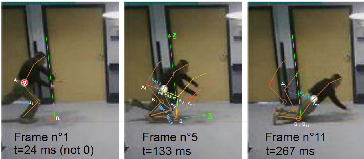
Figure 4.3.3: Kinematics of the fall via the images extracted from [Choi et al., 2015]
