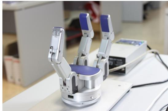
(c) The RBO Hand 2 gripper, that implements underactuation through compliant materials [53]. Picture: copyright ©2016, SAGE Publications
