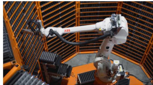
(d) Gripper constituted of two jaws used to pick battery cells [15]. Picture: copyright ©2021, ABB
