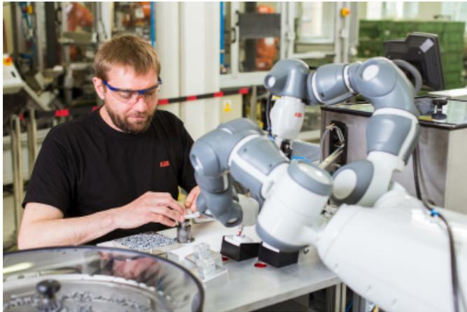
Figure 2 – A cobot collaborating with an operator for a small parts assembly task [16].
