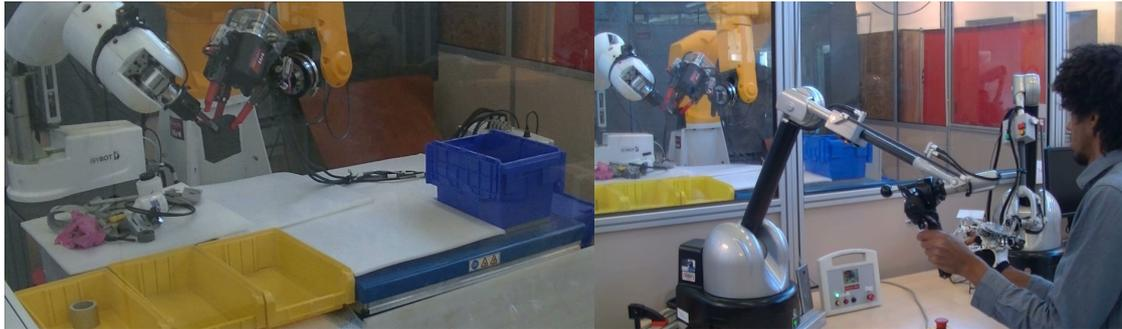
Figure 1.2 – ROMANS European project [30]. It aims at developing robotic solution for nuclear waste sorting and segregation. One of the proposed solution is a bi-manual master-slave tele-operated system.
