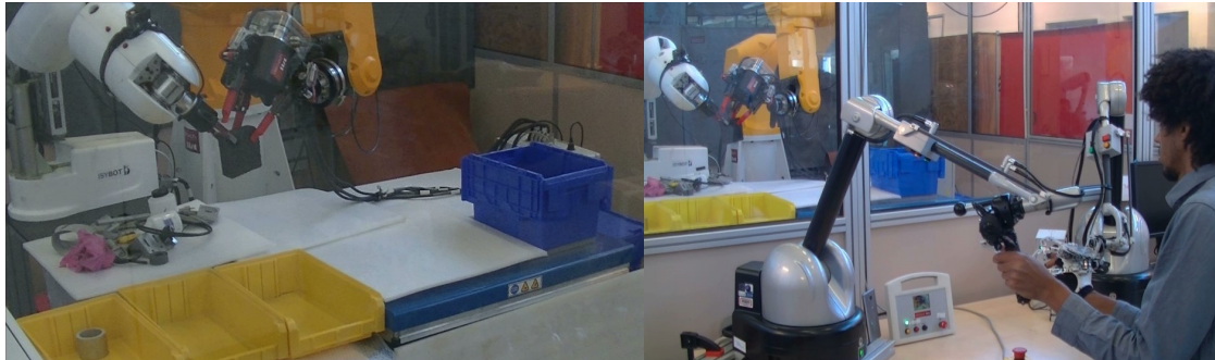
Figure 1.2 – ROMANS European project [30]. It aims at developing robotic solution for nuclear waste sorting and segregation. One of the proposed solution is a bi-manual master-slave tele-operated system.
