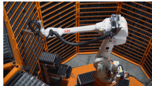
(d) Gripper constituted of two jaws used to pick battery cells [15]. Picture: copyright ©2021, ABB
