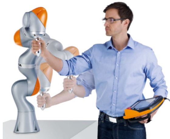
Figure 5 – Use of a collaborative robot to specify primitive grasps. When in gravity compensation mode, the operator is able to move the robot arm end-effector in any desired configuration (here with a Kuka iiwa): it could be used to set the primitive grasps. Picture: copyright ©2022 KUKA.
