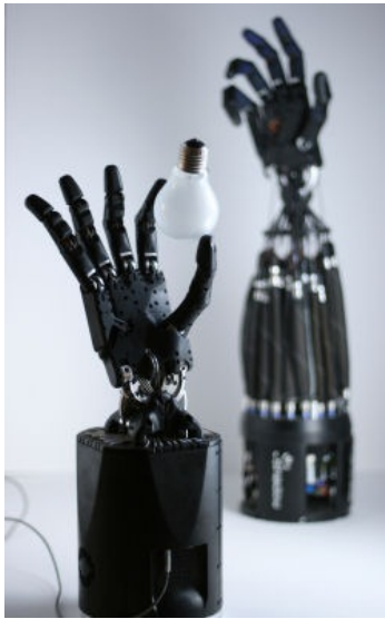
(a) ShadowHand gripper: 5 fingered gripper with 24 degrees of freedom. Picture: CC BY-SA license [44]
