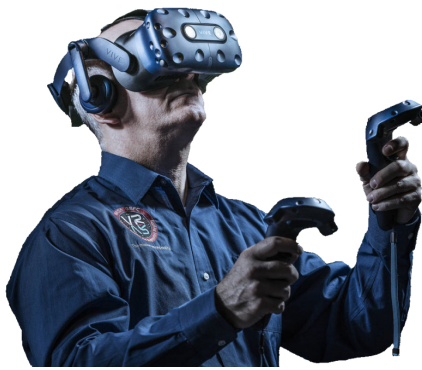
(a) Example of a virtual reality setup: a headset and two controllers with motion tracking. The controllers allow to interact with the virtual environment, for example to control the desired pose of the gripper. Picture: CC BY license [189]
