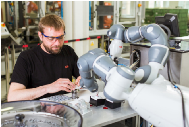
Figure 2 – A cobot collaborating with an operator for a small parts assembly task [16]. Picture: copyright ©2021, ABB
