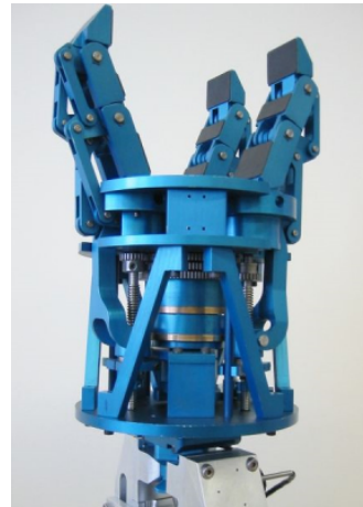
(b) The SARAH Gripper, an underactuated gripper based on differential mechanisms [51]. Picture: copyright ©2022 Université Laval [52]
