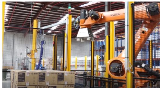
(c) Robot used in a palletizing system equipped with a suction gripper with four suckers [14]. Picture: copyright ©2021, KUKA
