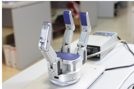
(d) The BarrettHand [6], an underactuated gripper using triggered mechanisms. Picture: CC-BY license [54].
