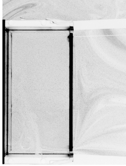
Figure 4.13: Example of a photo taken in the PIV measurement, in inverted colour (black turns to white and vice versa), 1 pixel equals to 0.082mm. Black points indicate the positions of tracers, which are almost uniformly distributed in the whole cavity.
