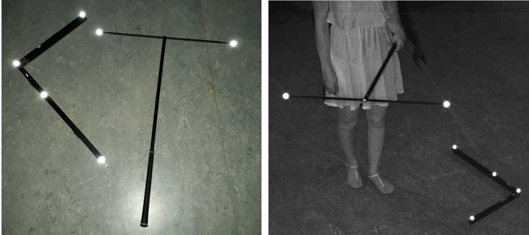
Figure 5.5: A subject sweeping the zone that needs to be covered by the Qualisys cameras using the calibration kit: the L-shaped reference structure and the calibration wand
