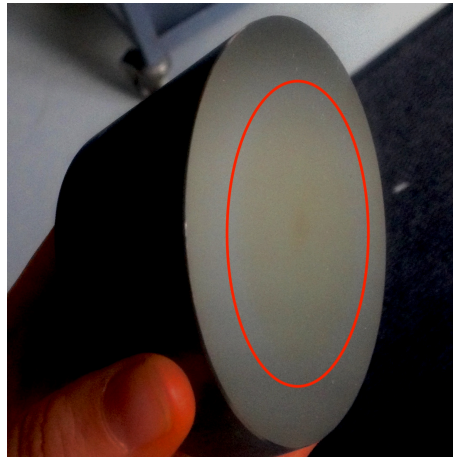
Figure 3.13: Picture of the dark stain on the first mirror. The stain is encircled in red. The contrast has been optimized in order to make the spot more visible. In real light, the spot is slightly less visible.
