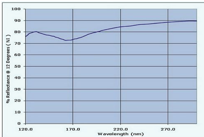
Figure A.8: Reflectivity as a function of wavelength for the eSource Optics Al/MgF 2 coating. Credit: eSource Optics.
