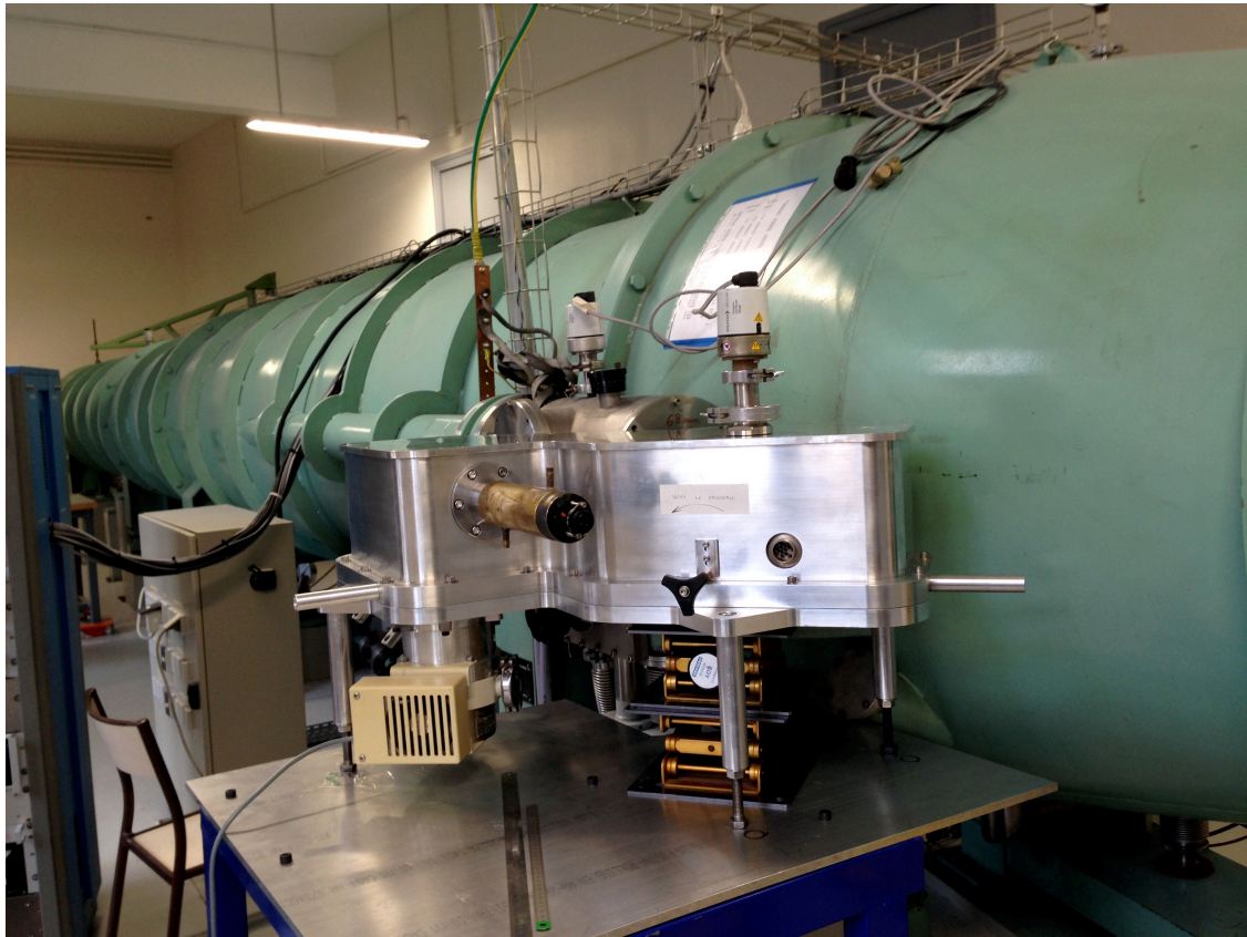
Figure 3.9: Picture of the spectrometer with the test bench at the input. The spectrometer is the green chamber, the test bench is the aluminum chamber in the foreground.
