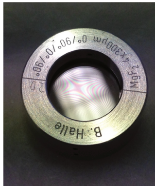
Figure 3.46: Sample E after cycles #3 to #10. Fringes are clearly visible. At least one of the 3 molecular bonding of sample E broke.
