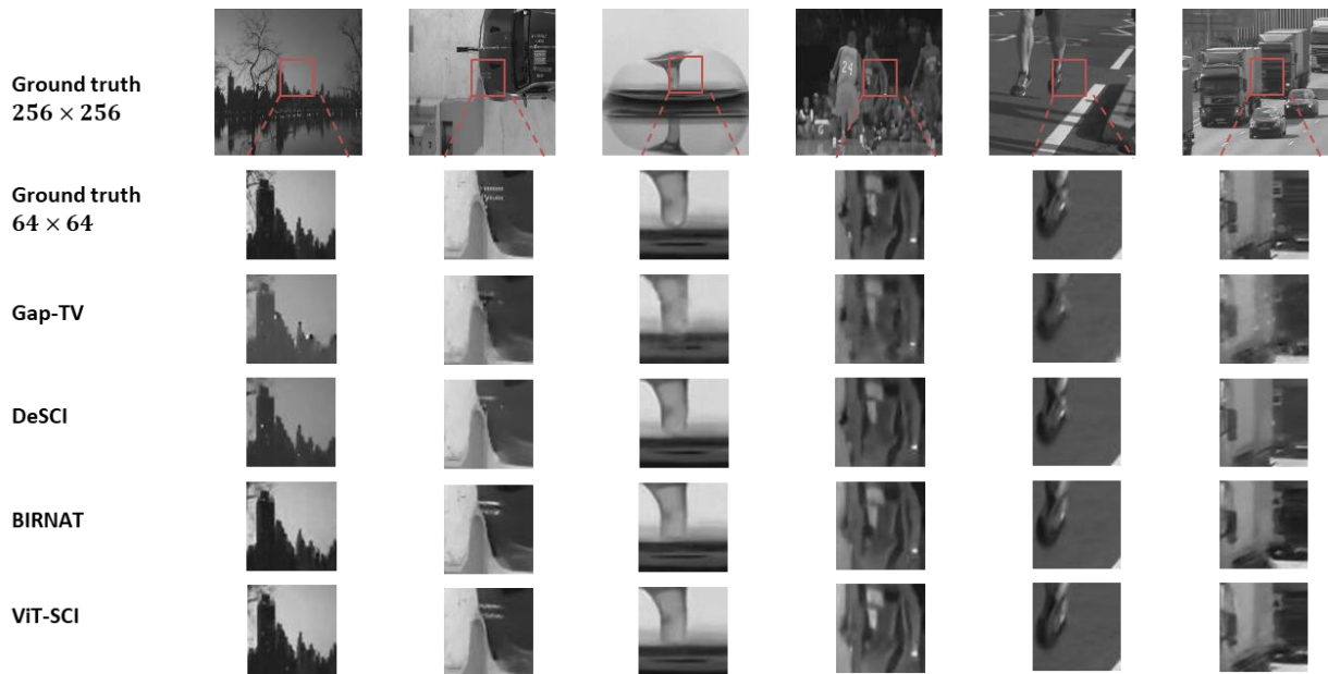
Figure IV.16: Reconstructed frames of GAP-TV, DeSCI, E2E-CNN, BIRNAT and ViTSCI on six simulated video SCI datasets.
