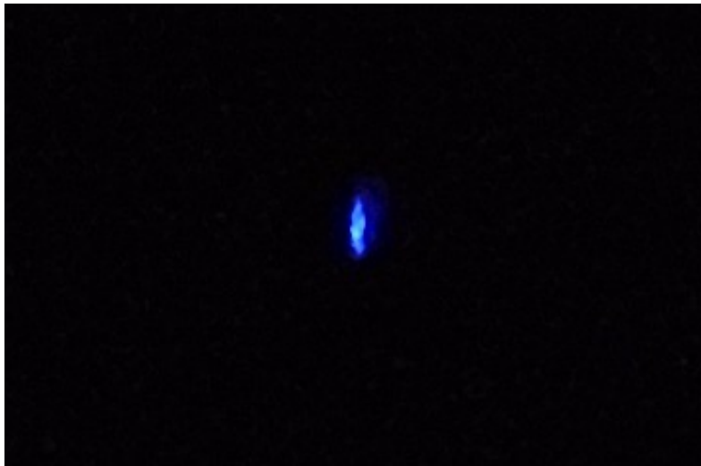
Figure 6.5: First image of the Cherenkov emission on the screen station TL/DG/SST.01 take the 21 st of July 2022. The image have been made with a phone camera at the exit of the accelerator bunker.
