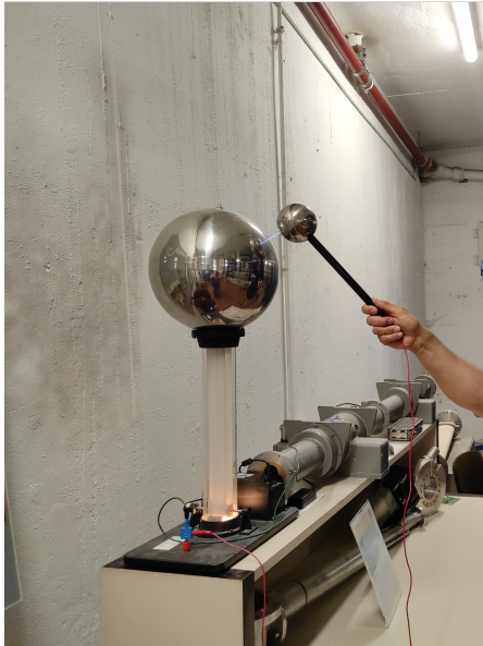
(a) The small Van der Graaff generator used at the museum "Science ACO" (Orsay, France) to create high voltage and demonstrate air breakdown.
