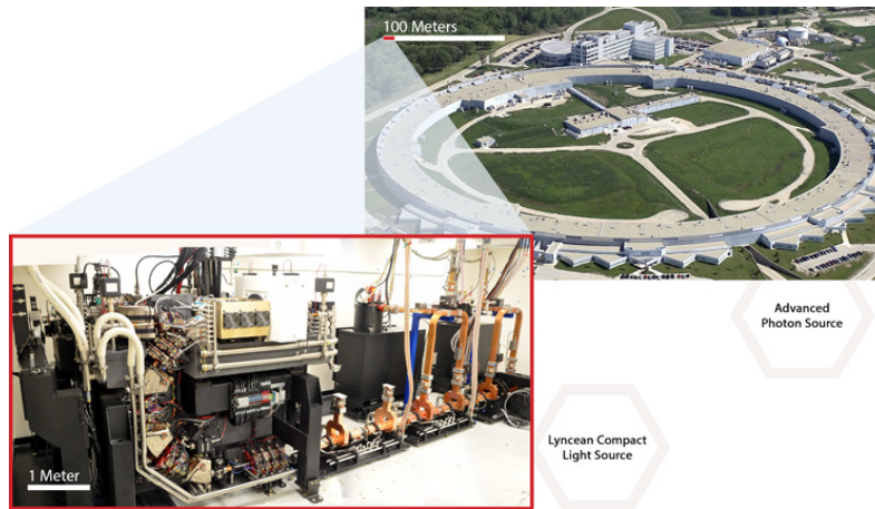
Figure 1.23: Comparison of Lyncean compact light source (CLS) and conventional synchrotron light sources [27].
