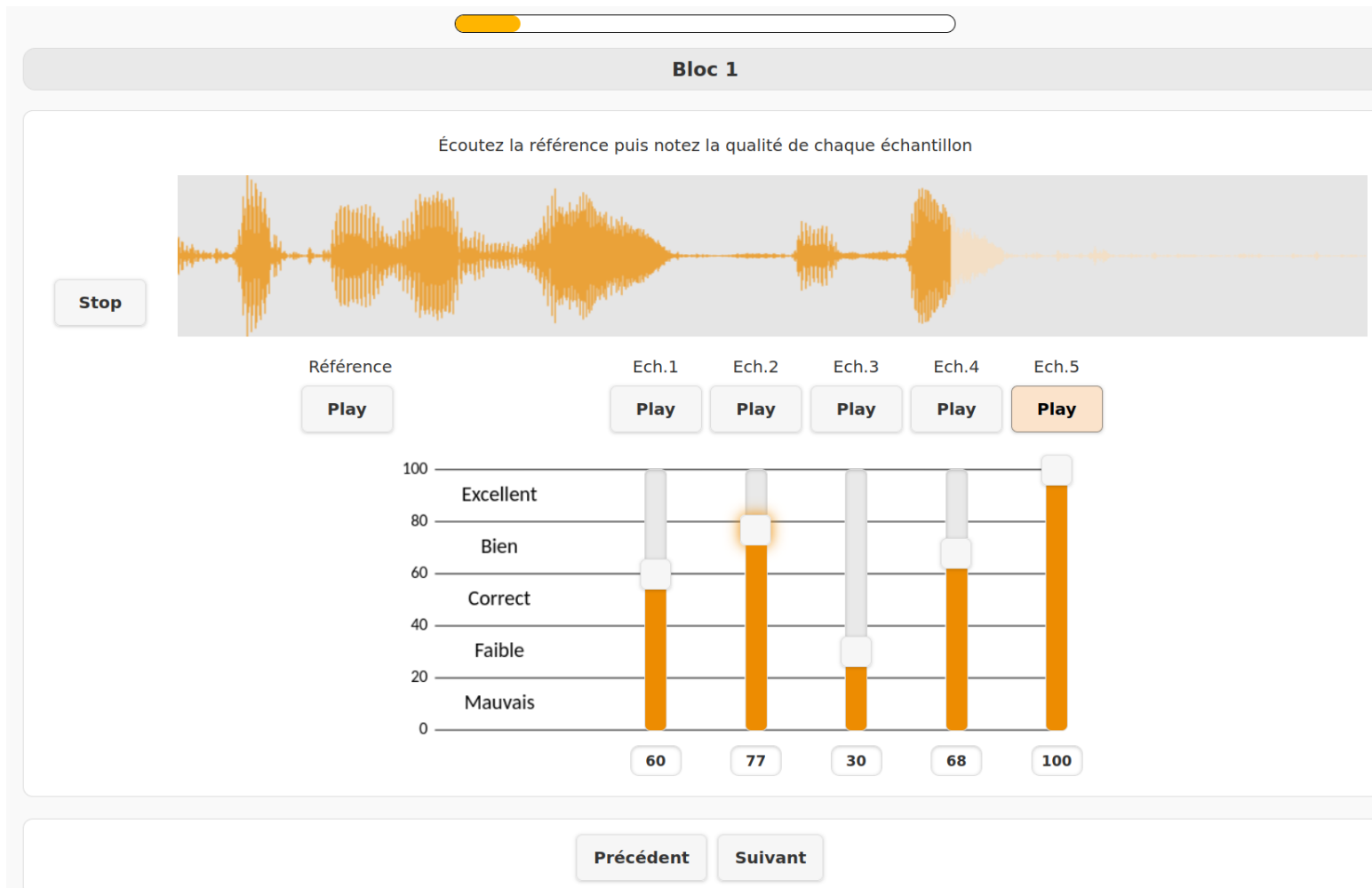
Fig. 3.14.: Online MUSHRA listening test. Screenshot of the web implementation of the MUSHRA test during the rating of an item. Reference and stimuli can be freely listened to by pushing the corresponding play button. The sliders are used to rate each stimulus compared to the reference.
