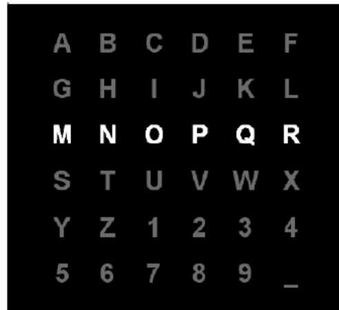
Fig. 1.20.: Display of a P300 Speller. One row or column is flashed at a time while the subject focuses on a single character. In this particular example, the line starting with M is currently intensified. from Schimpf and Liu, 2013
