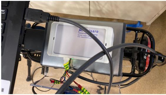
Figure 3.6. The data logger, IMU and GPS.
