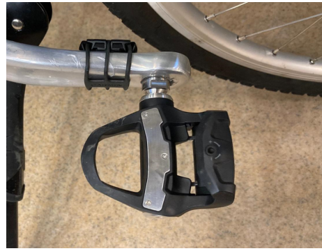
Figure 3.9. Power meter pedal+cadence sensor.
