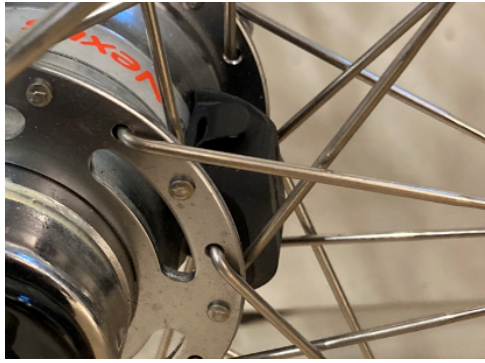
Figure 3.8. Garmin speed sensor fixed on the rear wheel hub.
