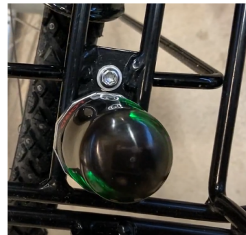
Figure 3.3. G-link-200 Triaxial accelerometer.
