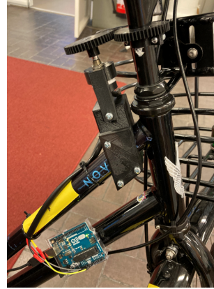
Figure 3.5. The potentiometer connected to Arduino micro-controller.
