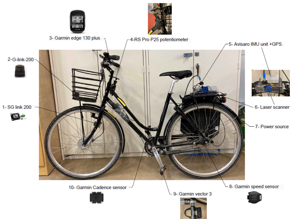
Figure 3.1. Schematic of the instrumented bicycle, more details about the different sensors following the correspondent numbers below.
