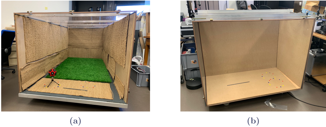
Figure 4.1 Photographs of the scale models of the rooms: (a) Main room and (a) reverberation chamber.
