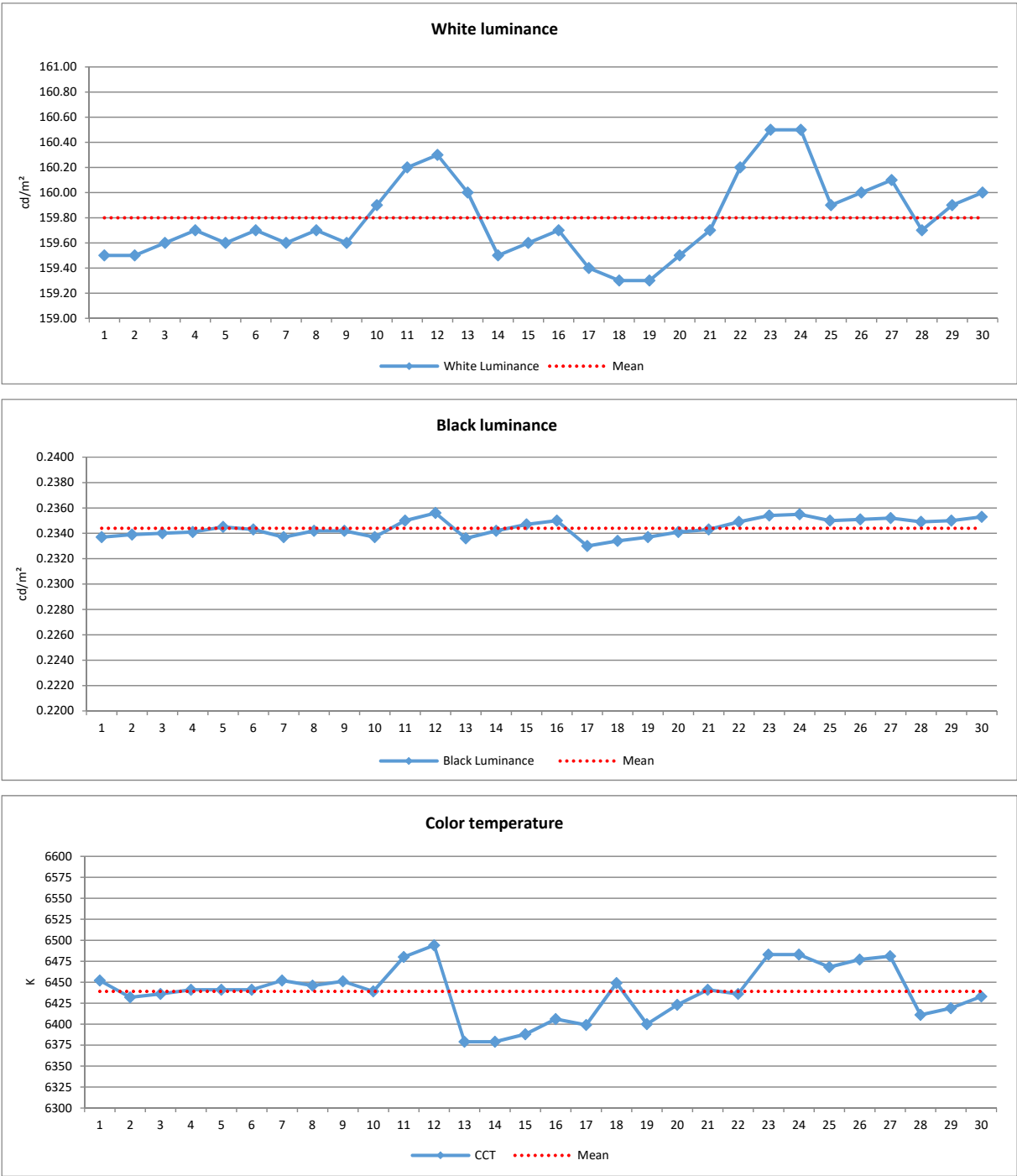
Figure 40. Measured values from 30 measurements in the defined test period of five days for Display 1.
