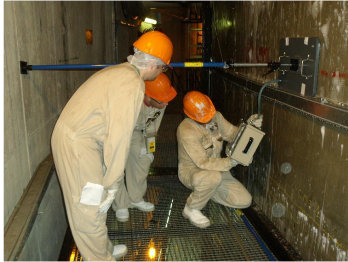
Figure 4.10: Measurement of local leaks during a pressurization test with a leakage collecting box, from (Asali, 2016).
