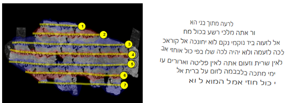
Figure 9.5: Imageline to textline alignment result as displayed in eScriptorium. Baselines are depicted in yellow, boundary polygons in alternating red and blue.
