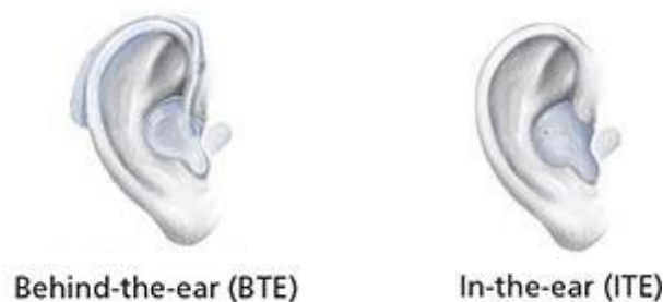
Figure 1.10. The two major classes of hearing aids: Behind the ear (left) and In the ear (right), adapted from 87
