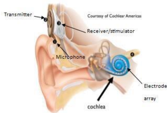
Figure 1.11. Main components of a cochlear implant inserted in a human ear: external parts comprises (1) microphone and (2) transmitter, internal parts comprises (3) receiver/stimulator and (4) electrode array inside the cochlea, adapted from 89
