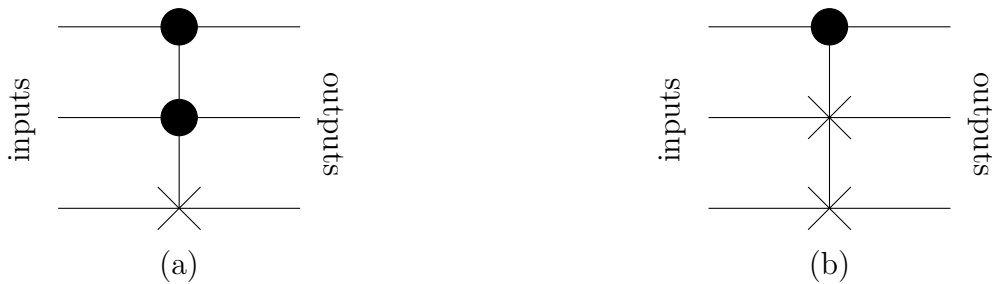
Figure 2.1: (a) Toffoli and (b) Fredkin reversible gate schemes. The black circles stand for the control bits, and crosses for the target bits.
